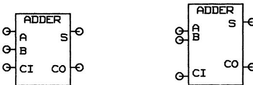
**Figure 4-14. Versions 1 and 2 of FULL ADDER.BODY**
