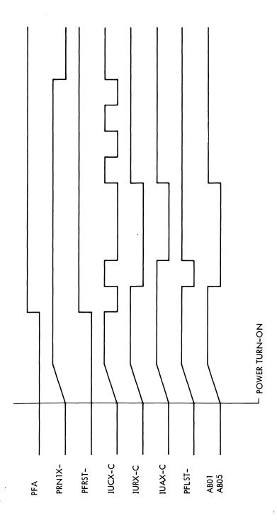
Figure 4-3. Power-Up Timing
