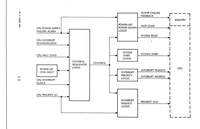
Figure 1-1. Power Failure/Restart Block Diagram
