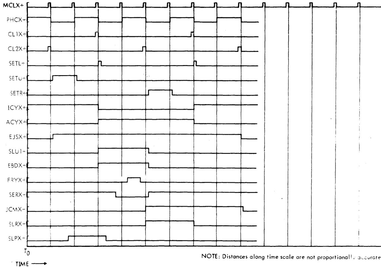
Figure IX-31. Sense (With Response) Timing
