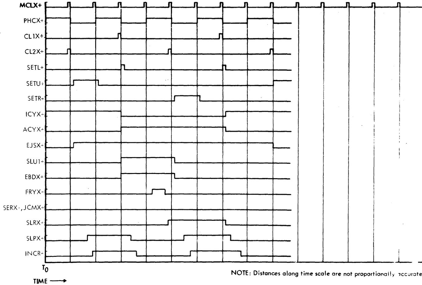
Figure IX-32. Sense (No Response) Timing
