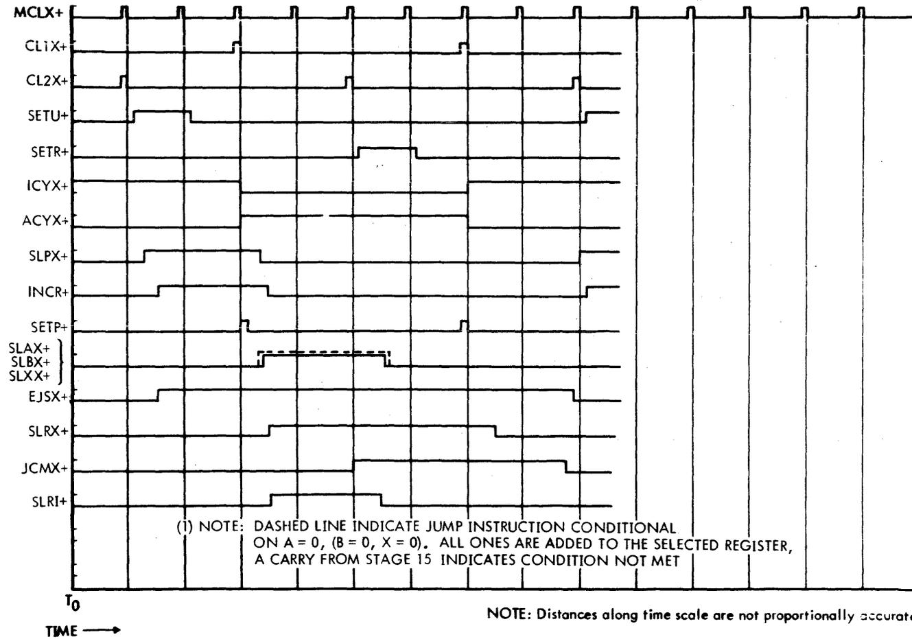
Figure IX-26. Jump Condition Met Timing
