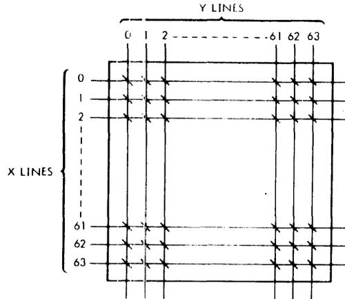
NOTE: A SENSE/INHIBIT LINE, NOT SHOWN ABOVE, ALSO PASSES THROUGH ALL CORES OF A 4K MAT PARALLEL TO THE X LINES.
