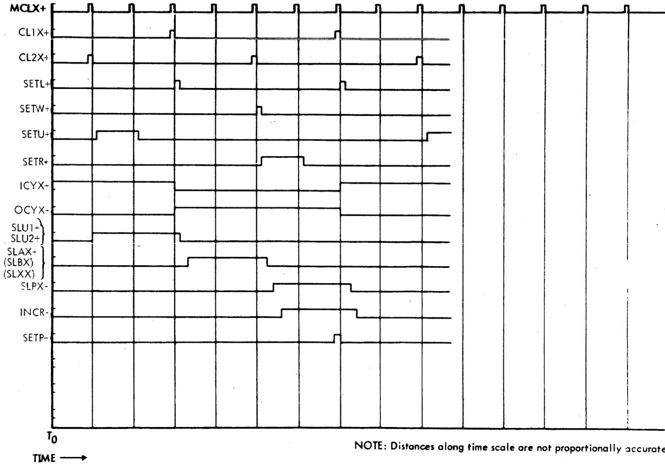
Figure IX-18. Store A (B, X) Register Timing
