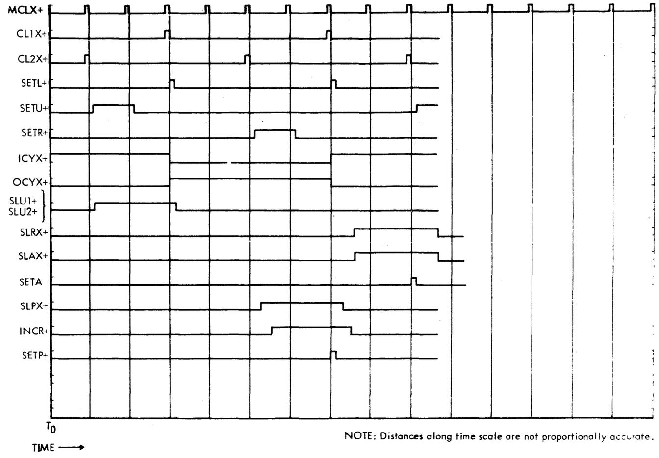
Figure IX-20. Add To A Register Timing
