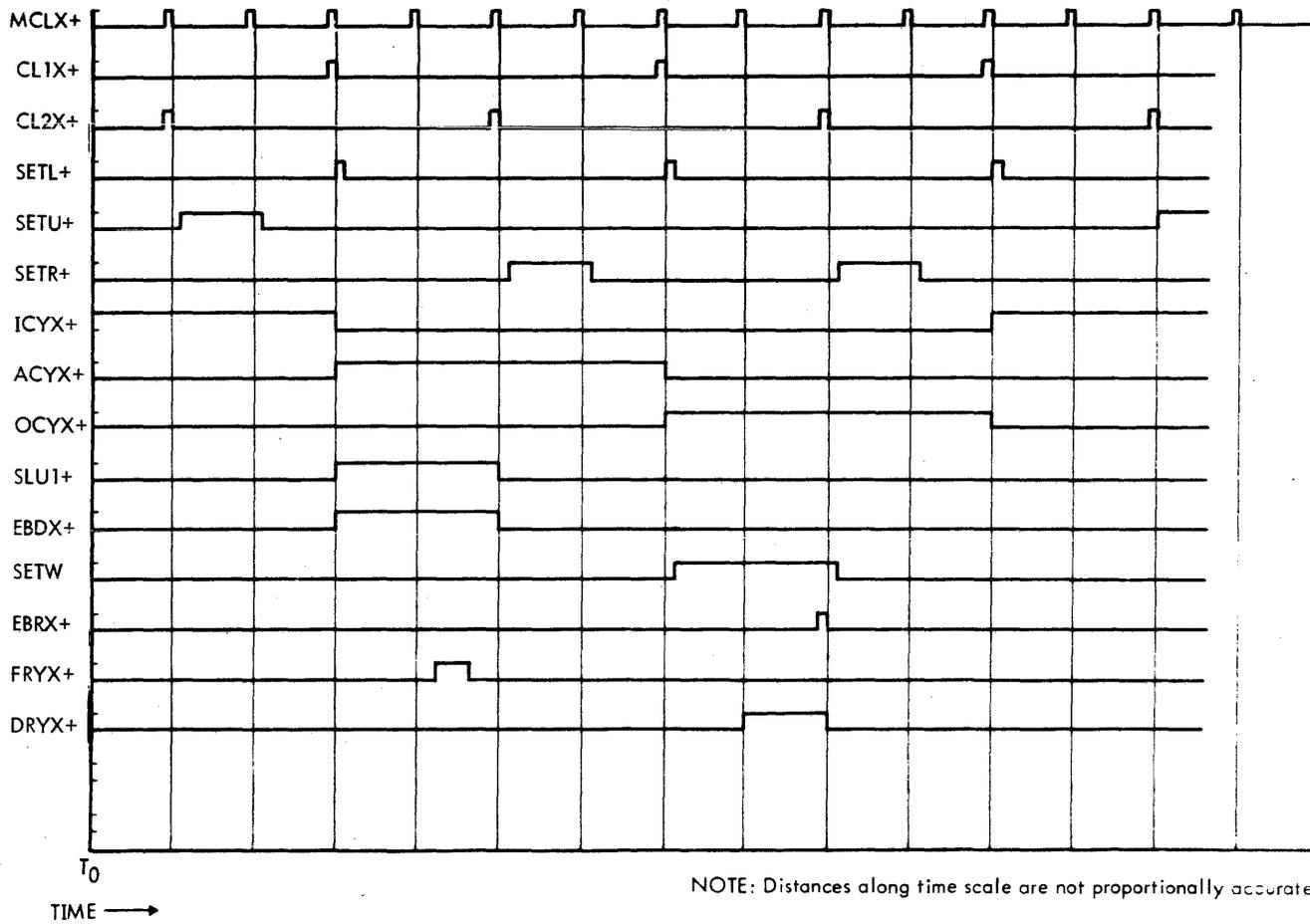
Figure IX-34. Input To Memory Timing
