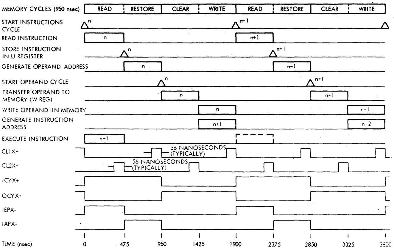
Figure IV-17. Sequence For Operand Storage In Memory
