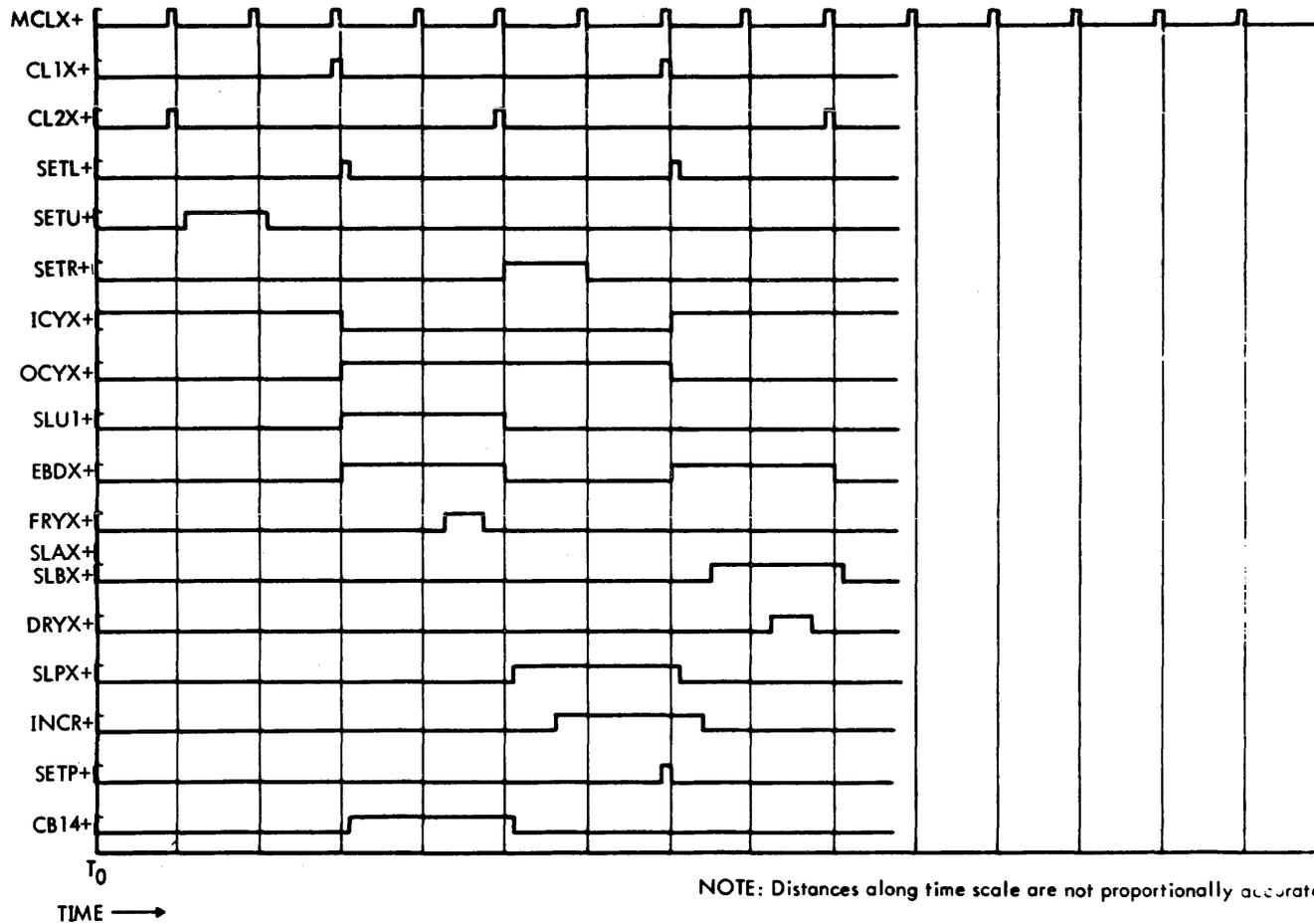
Figure IX-35. Output From A, B Register Timing
