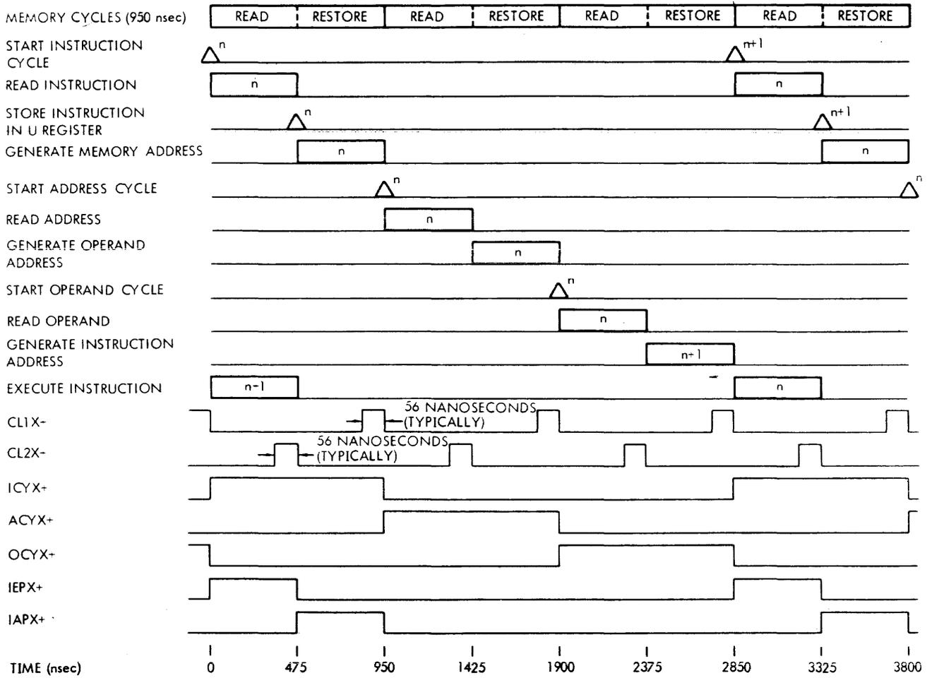
Figure IV-18. Sequence For Indirect Operand Access
