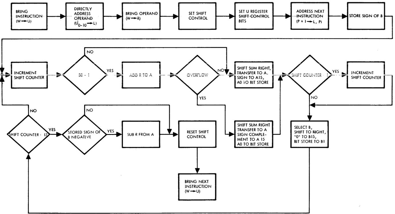
Figure X-4. Flow Diagram of the Multiplication Instruction
