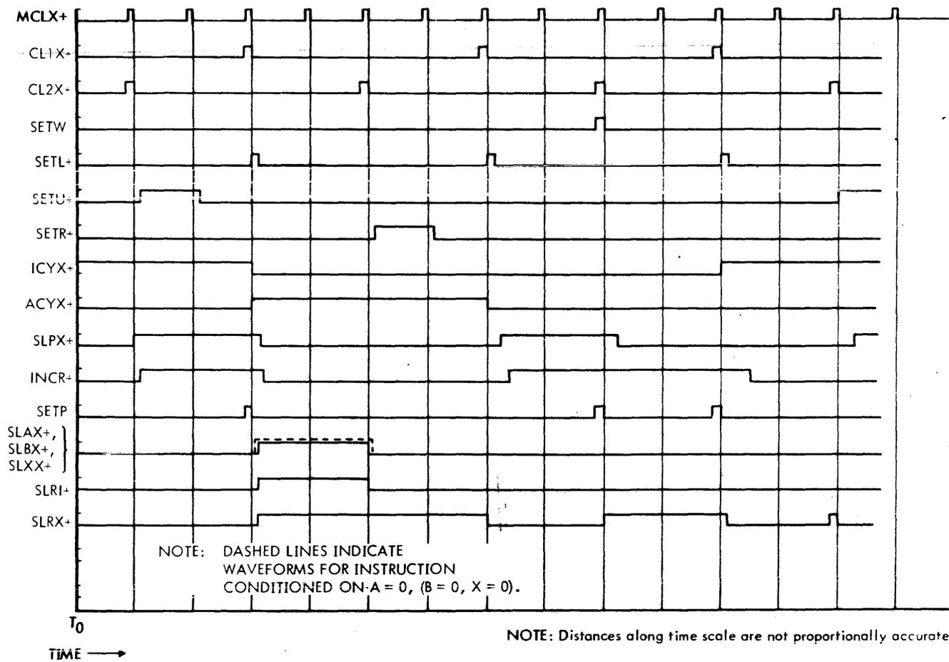
Figure IX-27. Jump-and-Mark Condition Met Timing
