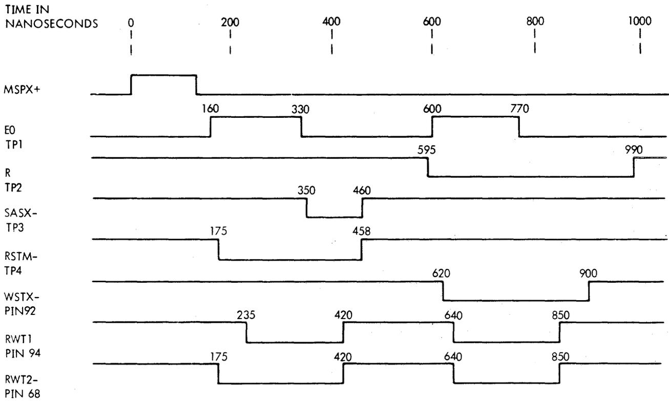
Figure V-18. Test Point Waveforms on Timing and Control Card
