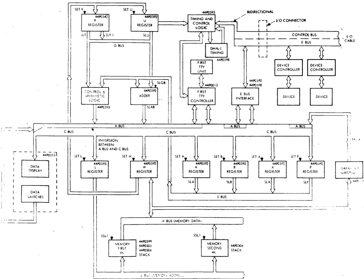
Figure IV-1. 620/L CPU Block Diagram
