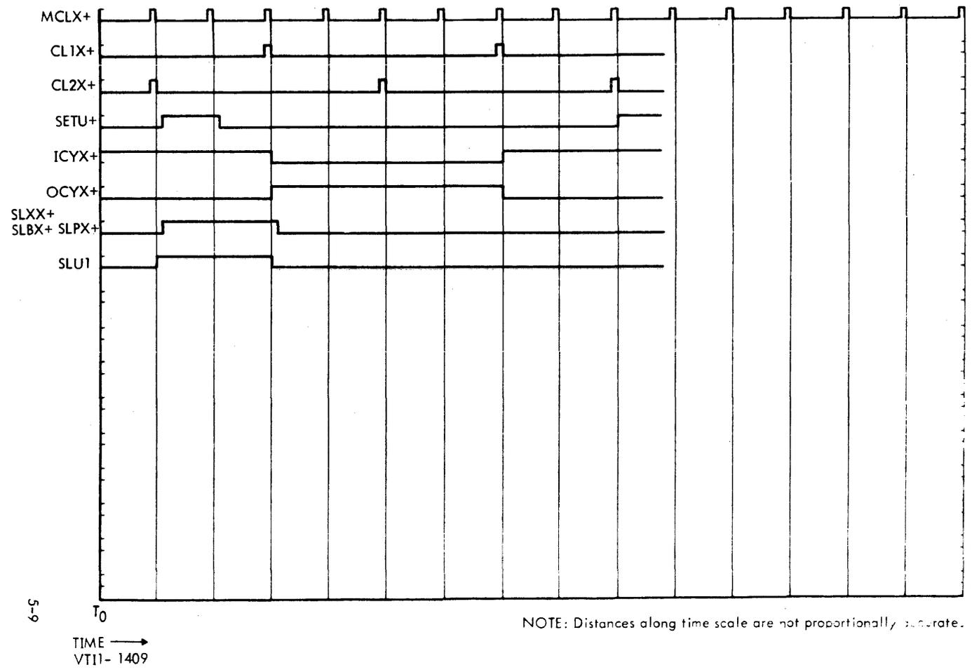
Figure IX-6. Index and Relative Addressing Timing
