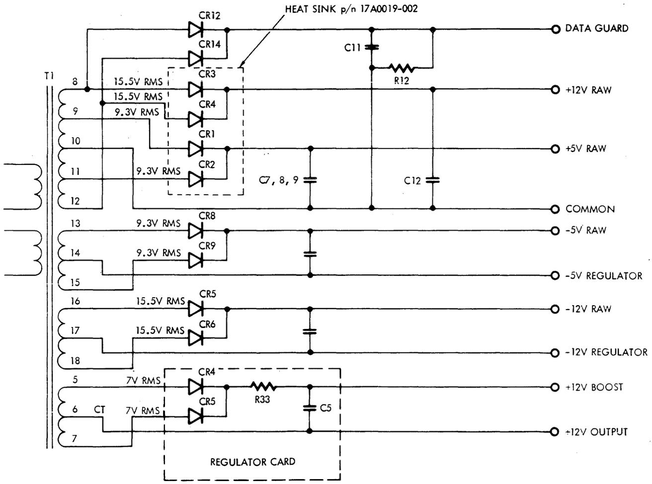
Figure VII-3. Rectifier and Filter Circuits
