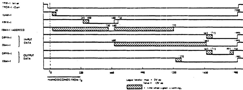
Figure 8-12. DMA Input and Output Timing
