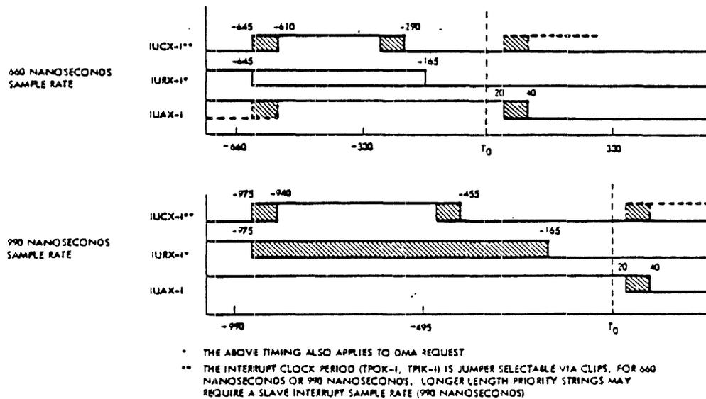
Figure 8-13. DMA and Interrupt Request Timing
