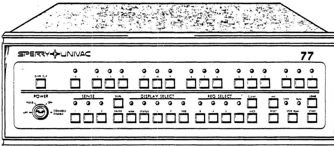
Figure 2-1. The V77-600 Mainframe (7-inch Chassis)
