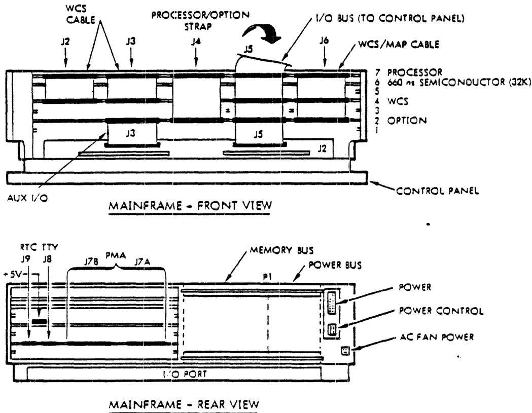
Figure 5-13. Typical Computer Installation with WCS
