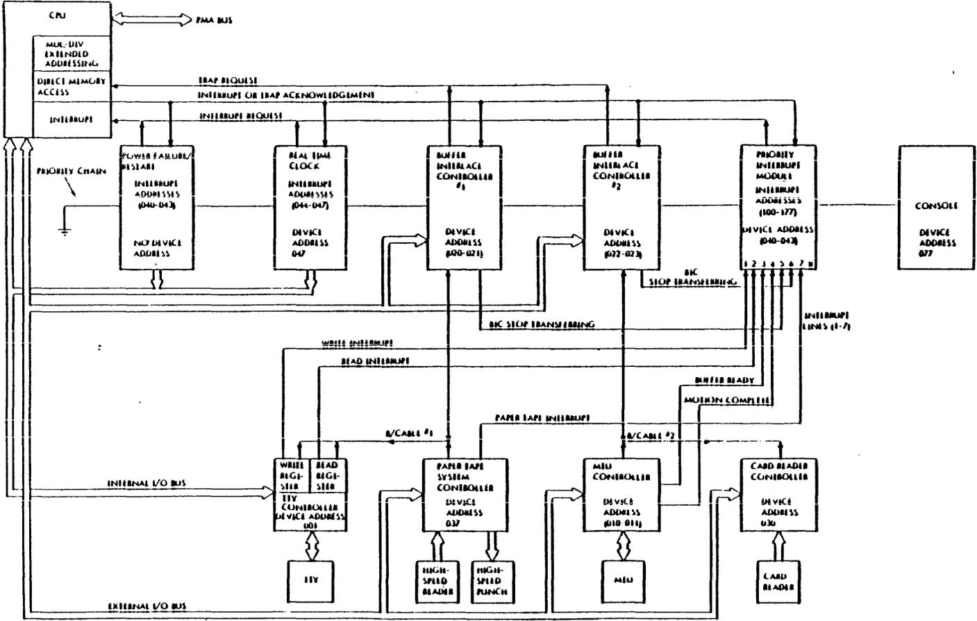
Figure 8-3. Typical I/O System Block Diagram
