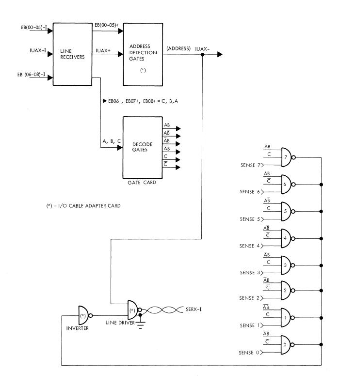
Fig. 2-9 Example of Sensing Eight Sense Lines
