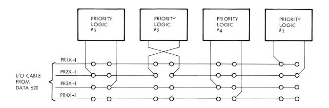
Fig. 2-15 Priority Assignment by Jumpers
