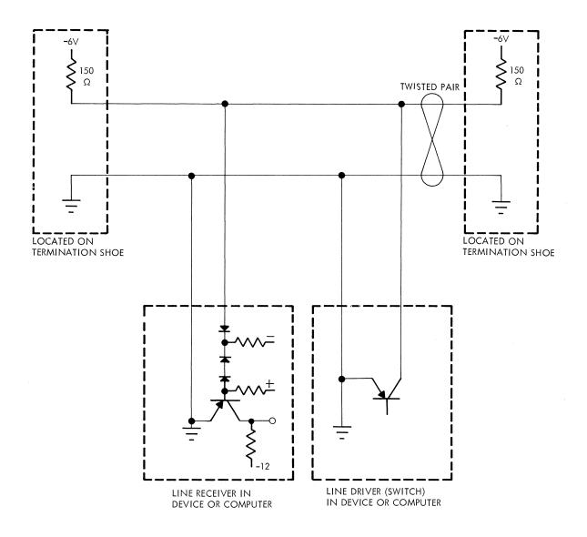
Fig. 2-4 Typical Line Location on I/O Bus
