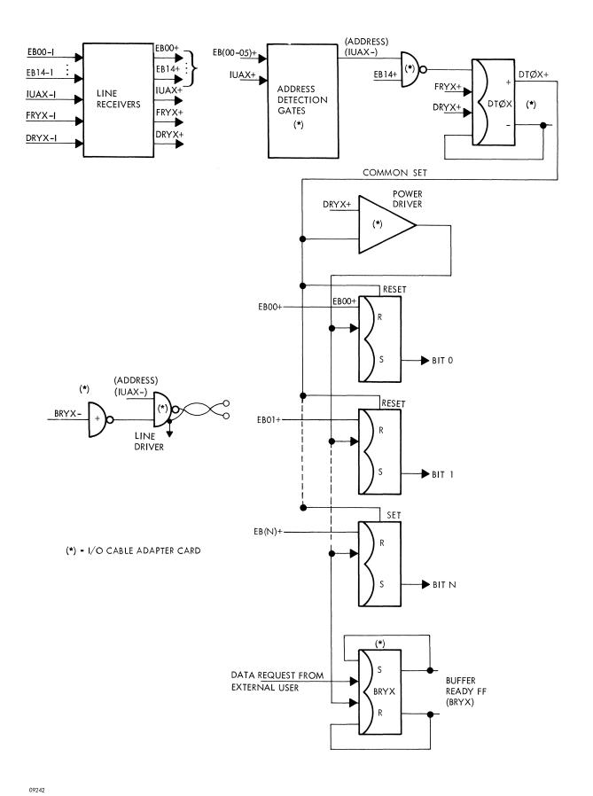
Fig. 2-13 Example of Buffer Data Transfer Out
