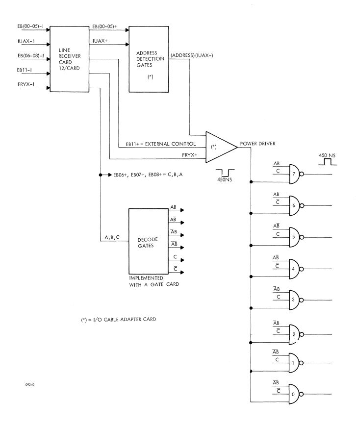
Fig. 2-7 Example of External Control for Eight EXC Lines
