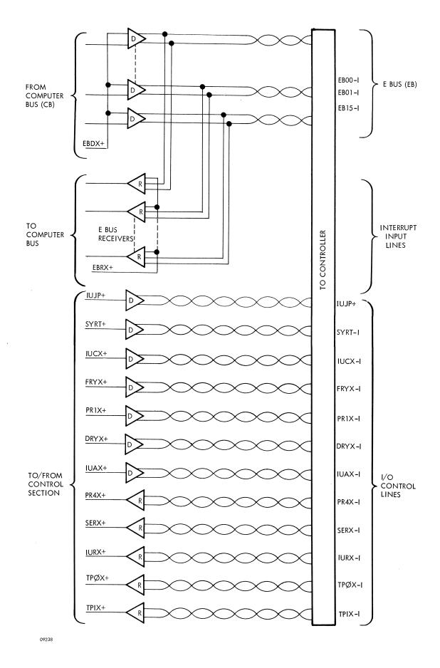
Fig. 2-3 DATA 620 I/O Section and Standard Connections
