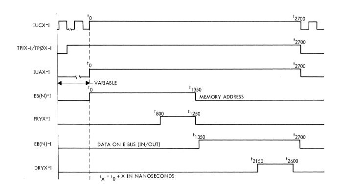
IUCX-I - REMOVED AT  $t_0$  RETURNS AT  $t_{2700}$ TPIX-I/TPØX-I - NORMALLY REMOVED AT  $t_{2700}$ , MUST BE REMOVED BY  $t_{2900}$ EB(N)-I ADDRESS - NORMALLY ON  $t_0$ , MUST BE ON  $t_{600}$ NORMALLY OFF  $t_{1350}$ , MUST BE OFF  $t_{1950}$ EB(N)-I DATA (IN) - NORMALLY ON  $t_{1350}$ , MUST BE ON  $t_{1900}$ NORMALLY OFF  $t_{2600}$ , MUST BE OFF  $t_{2900}$ EB(N)-I DATA (OUT) - WILL BE ON  $t_{1500}$ , WILL BE REMOVED  $t_{2700}$ NOTE SIGNAL INVERSION ON I/O LINES
