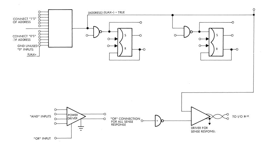
contain a device address, and bits EB06-08 indicate the particular function code for that device. EB11 is true indicating that an External Control Function is being performed (see Table 2-3). The pulse FRYX+ is used with the address to form a 450-nsec pulse for setting and resetting flip-flops. The address overlaps FRYX+ by 100 nsec to allow for logic delays in forming the pulse signal in the power drivers.
