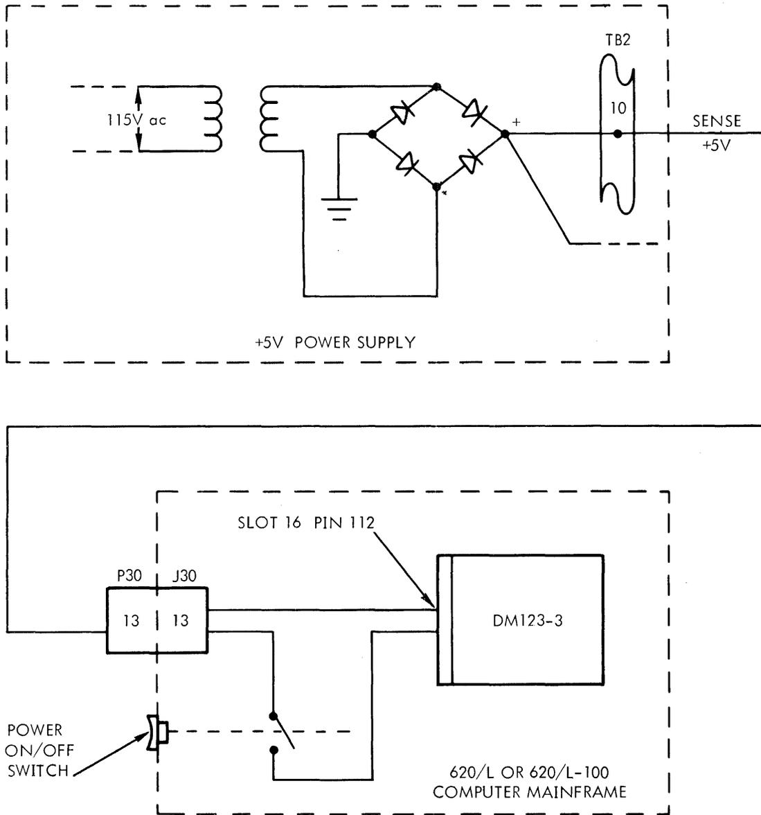
Figure 1-7. Source and Routing of Sense +5V
