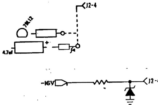
THE ZENER VOLTAGE WILL DEPEND ON THE KEYBOARD REQUIREMENTS IF IT IS NEEDED AT ALL, AND THE RESISTOR SHOULD BE SELECTED TO BIAS THE ZENER WITH AT LEAST 10MA OF CURRENT IN ADDITION TO THE CURRENT REQUIRED BY THE KEYBOARD.
