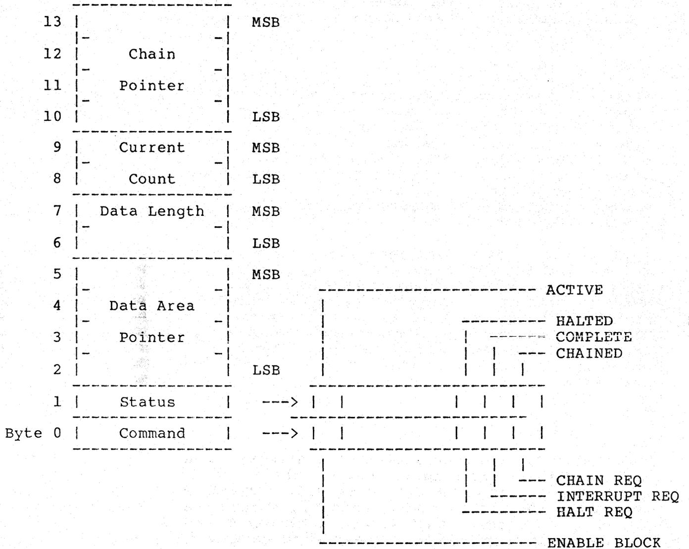
Figure 5.3 : DMA Block Header
