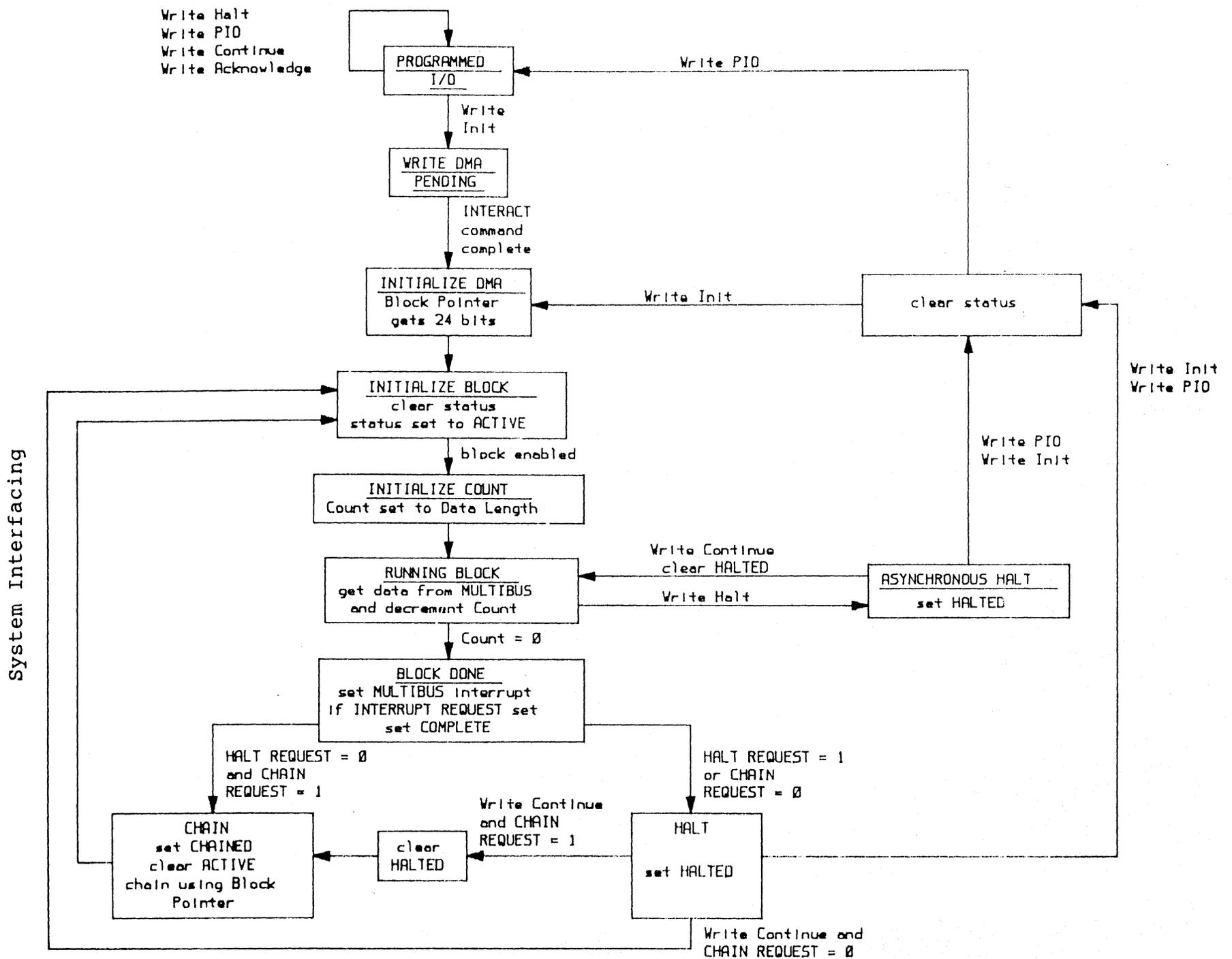
Figure 5.4 : DMA Write State Diagram
