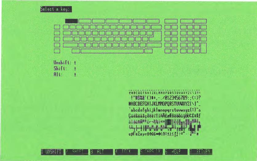
Below the keyboard, you'll see a display showing the status of the highlighted key in each of its modes (shifted, unshifted, and alternate). The values of each key are displayed to the right of the keyboard. The character set is displayed at the lower right.
