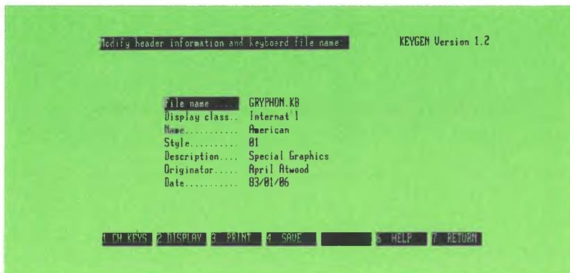
The keyboard file name and header information are displayed in the center of the screen. (Header information is the information about keyboard display class, name, date, and so on, located below the file name.) To change the file name or any header information, use the arrow keys to move the cursor to the desired line. The first data field (File Name) is displayed in reverse video, with its current value to the right of it. To change the value, type:
