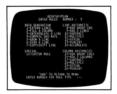
INSERT ADDITIONAL RULE allows you to add a new rule between two previously entered rules. Select Function 2 from the main ENTER RULES menu. You'll then be prompted for the rule number of this newly inserted rule. This number should be the number for the sequence in which this new rule is to be executed. (The rule which previously had this number, and all successively higher numbered rules will automatically be incremented by one after a rule is inserted.)
