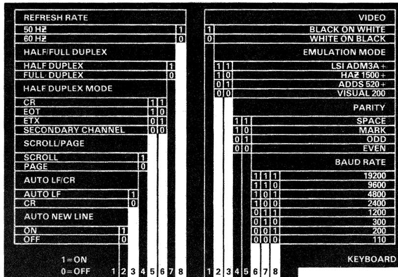
Figure 3-1 Rear Panel Switches
