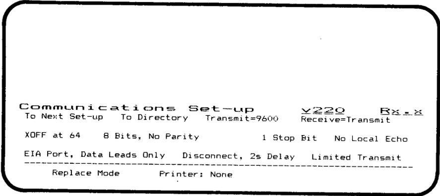
**Figure 3-6. Communications Set-Up Menu (with Default Values Displayed)**
