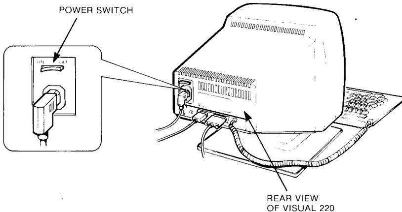
**Figure 2-1. The Visual 220 Terminal Power Switch**
