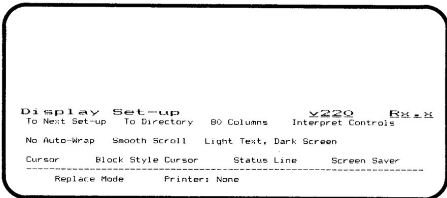
**Figure 3-4. Display Set-Up Menu (with Default Values Displayed)**
