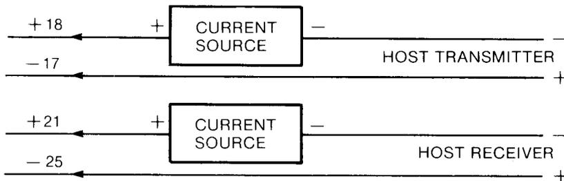
**Figure 5-2. Full Duplex 20 mA Current Loop Diagram**
