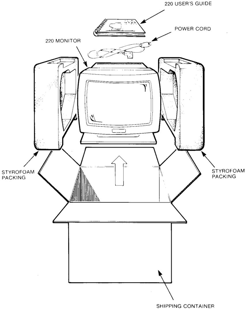
**Figure 4-2. Unpacking the Monitor Shipping Carton**
