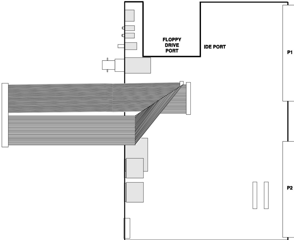
Figure 1. Connecting the Cable Assembly to the CPU
