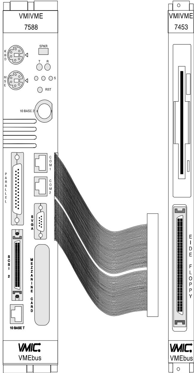
Figure 2. Connecting the CPU to the VMIVME-7453
