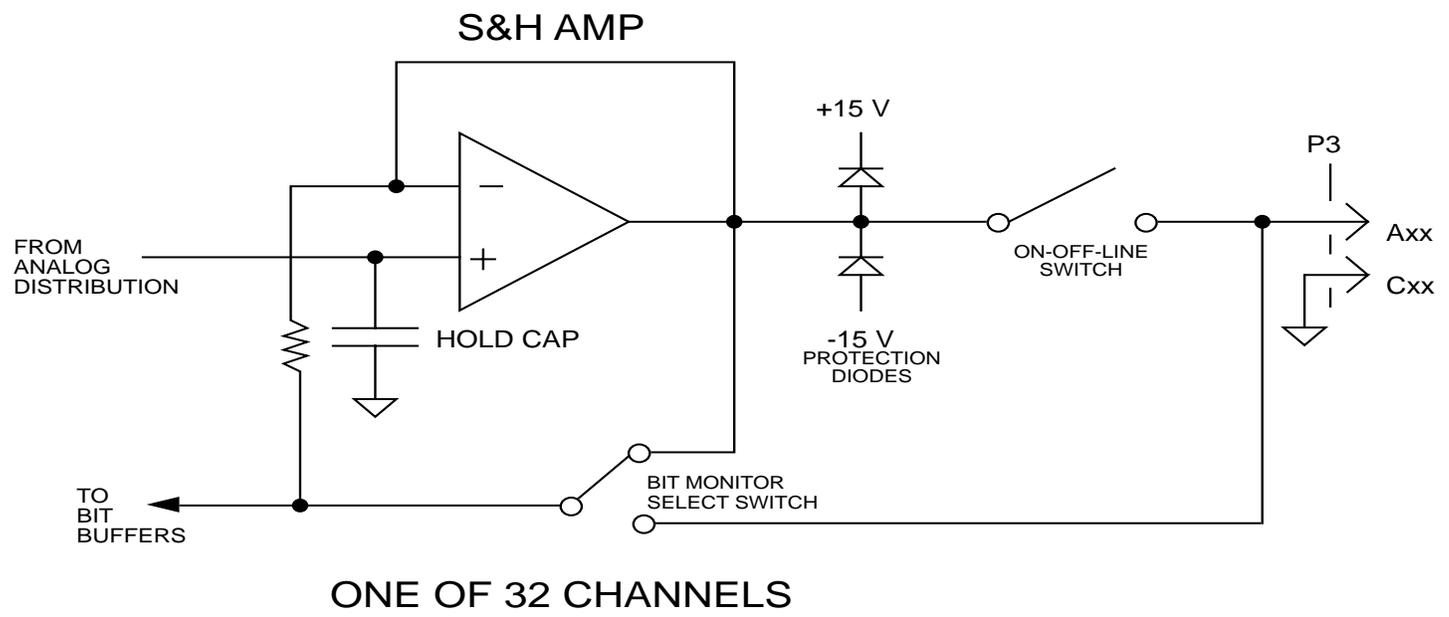
Figure 1-4 Simplified Output Buffers and Switches
