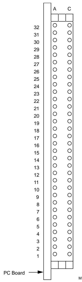
Figure 2-7 P3 Connector Pinout
