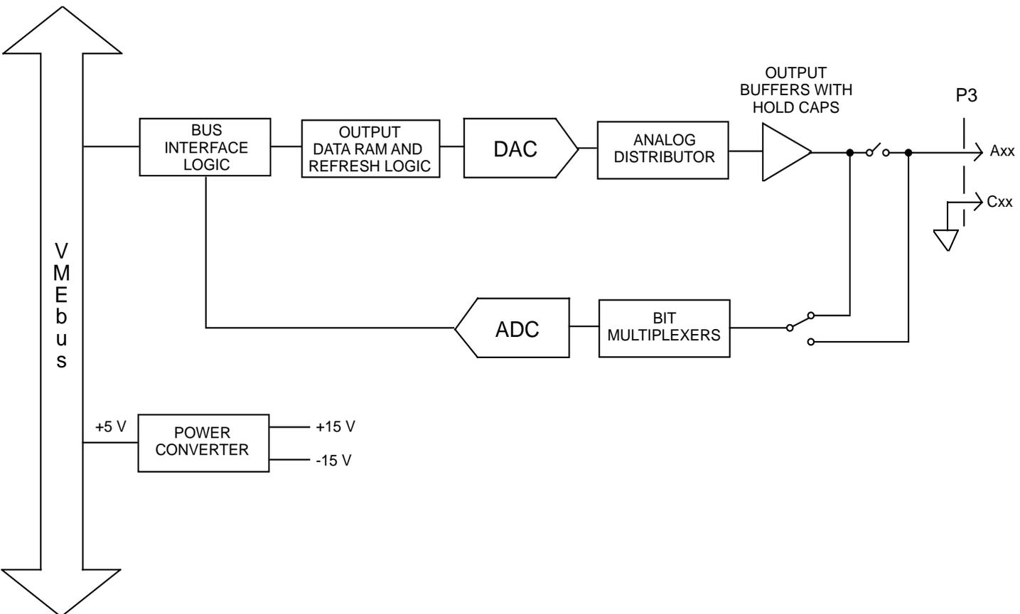
Figure 1 VMIVME-4132 Block Diagram
