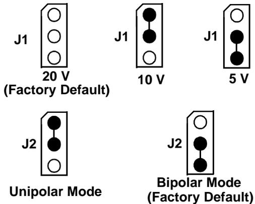
**Figure 2-4** Analog Output Voltage Range Selection
