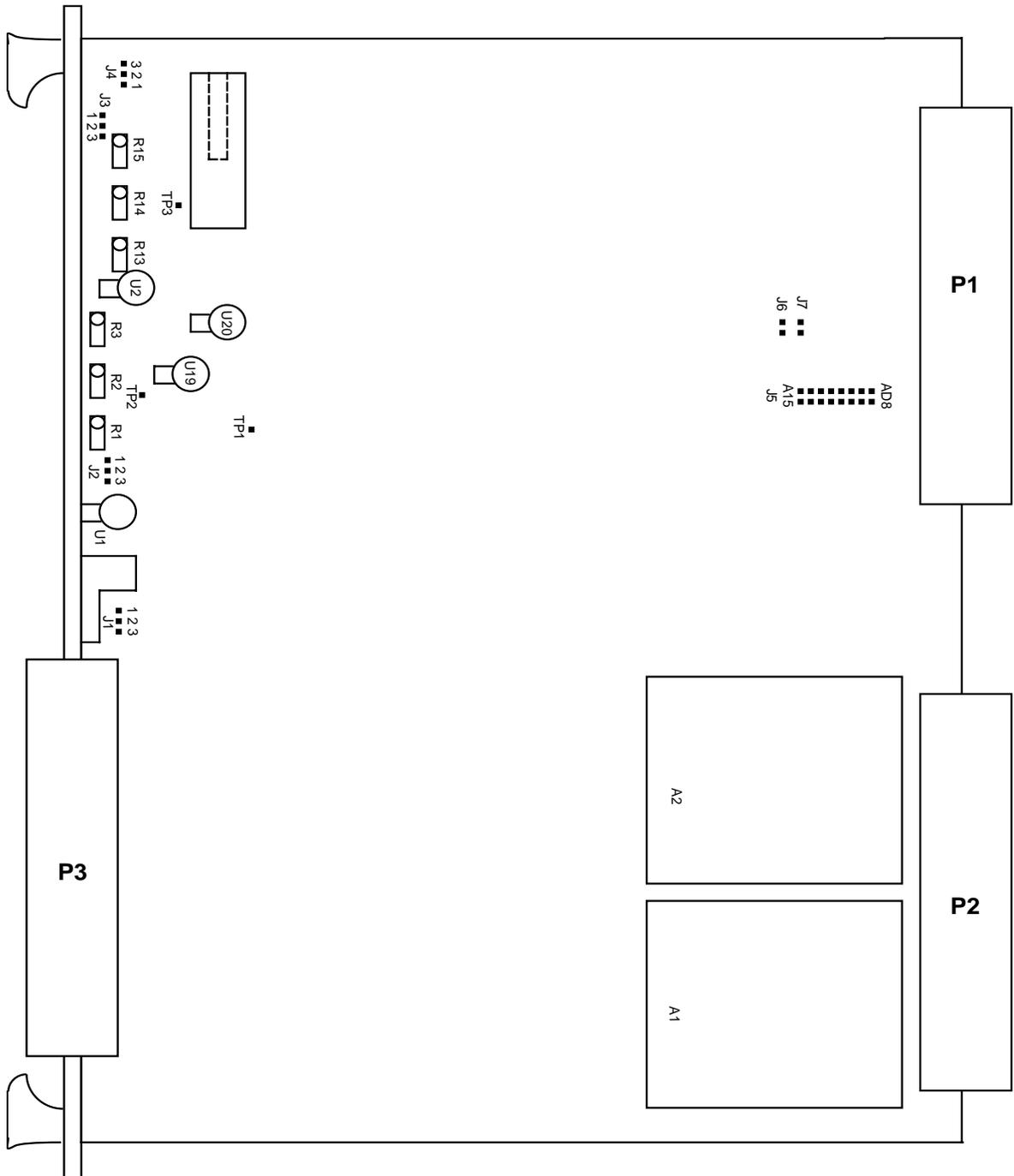
Figure 2-1 Jumper and Calibration Point Locations
