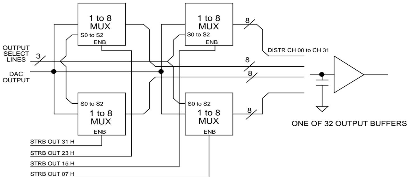
Figure 1-3 Analog Output Distribution
