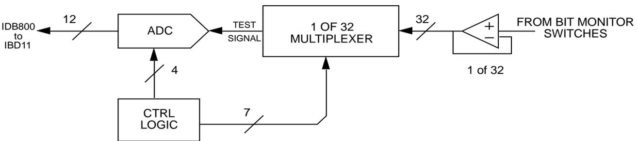
Figure 1-5 Simplified BIT Logic
