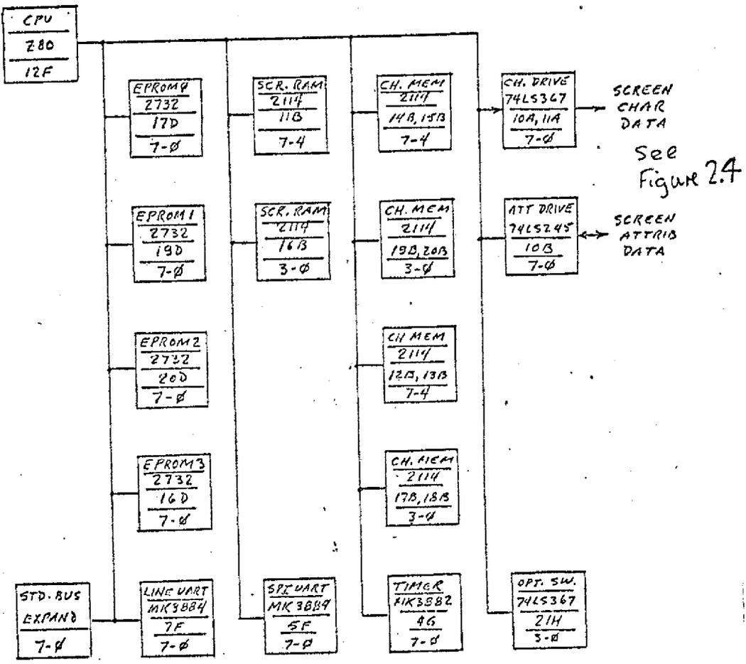
Figure 2.3 Block Diagram of the Data Bus
