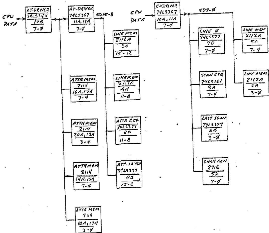
Figure 2.4 Block Diagram of the Screen Data Bus
