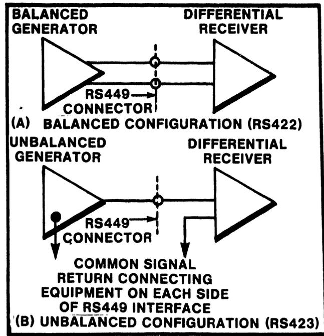
FIG. 2 RS449 INTERFACE CIRCUIT CONFIGURATIONS
