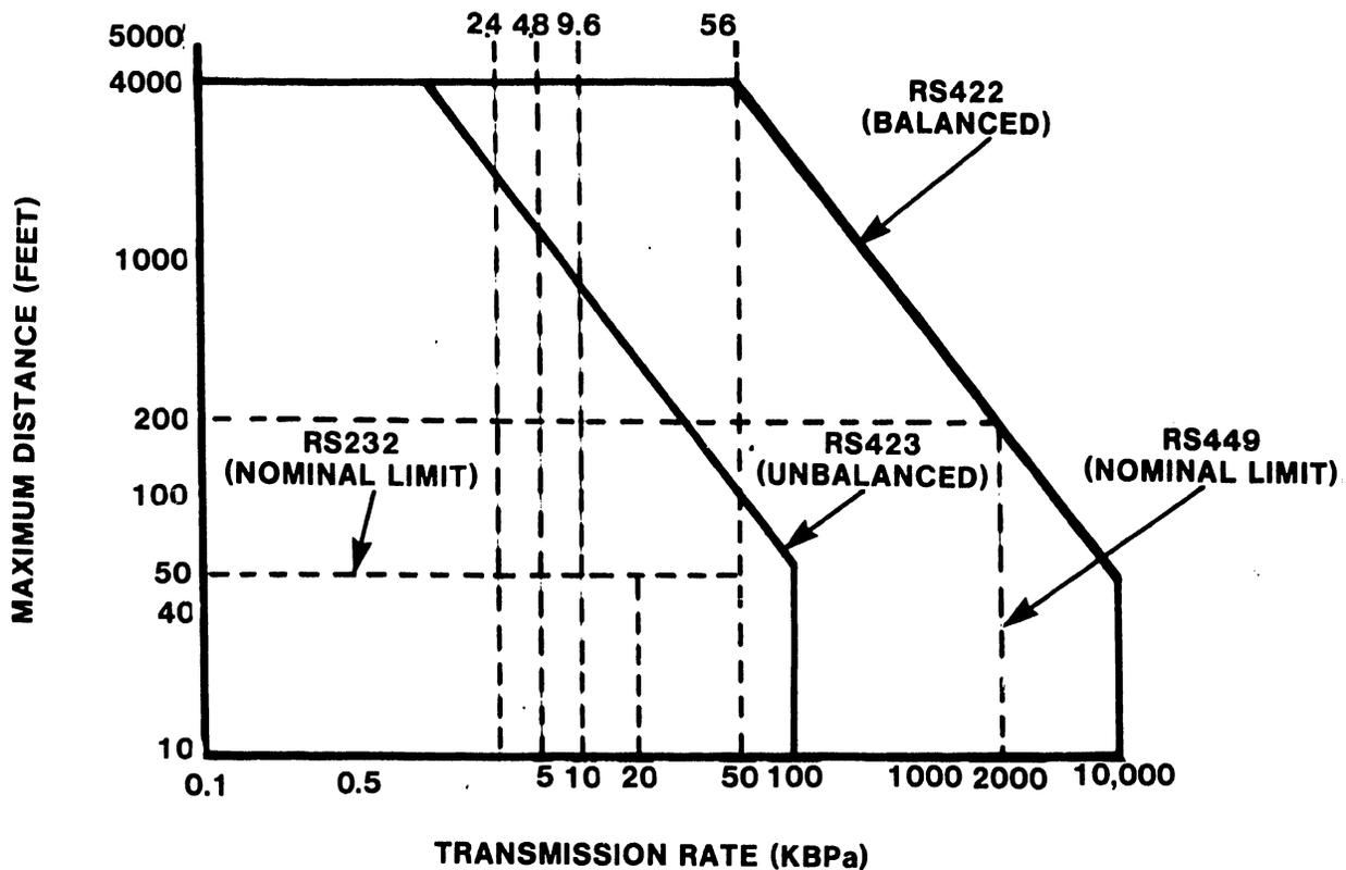
FIG. 3 PERFORMANCE PARAMETERS OF RS449 AND RS232 CIRCUITS
