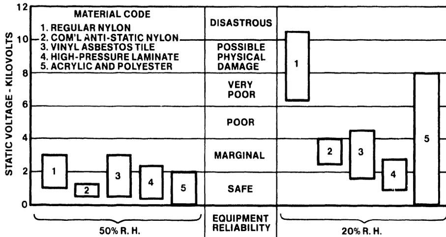
TYPICAL STATIC VOLTAGES GENERATED BY WALKING ON COMMON FLOOR COVERING MATERIALS
