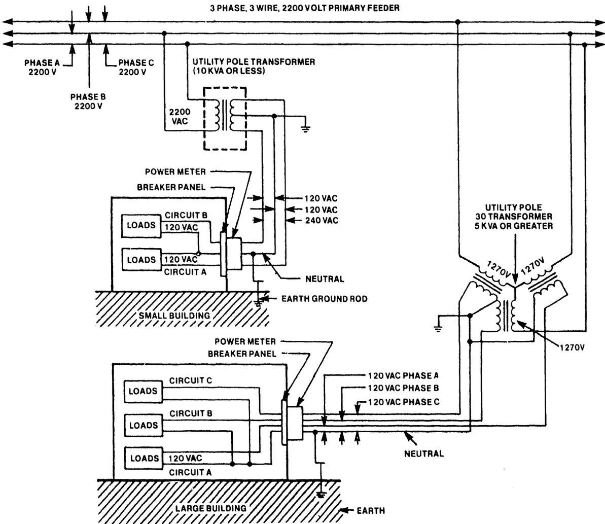
FIGURE 4-2 3-PHASE, 3-WIRE 2200 VOLT PRIMARY FEEDER
