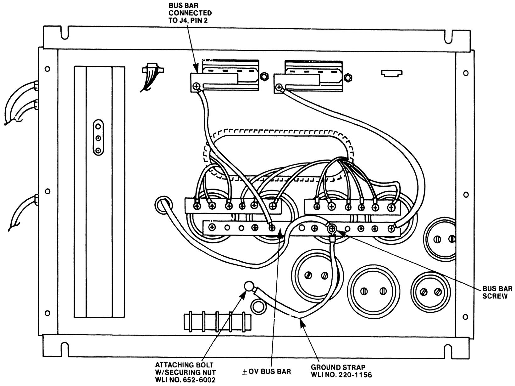
FIGURE 5-1 VS 60/80 POWER SUPPLY (Bottom View)
