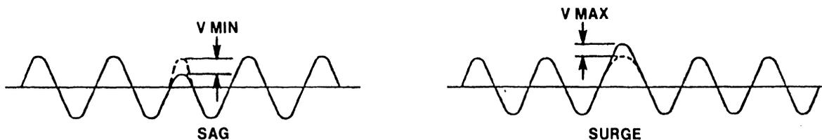
FIGURE 4-8 SAG AND SURGE WAVEFORMS
