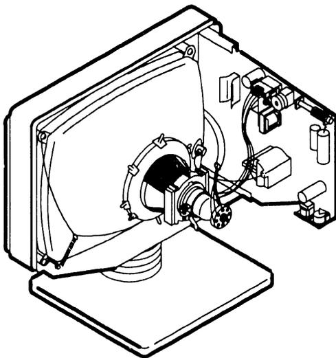
**11** Check top row of characters for distortion. Adjust R1 to remove distortion, if any.
