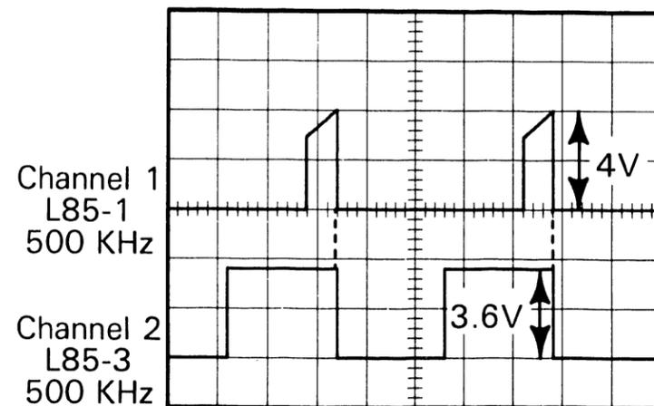
7 Transfer channel 1 of scope to L85-3 on RMU board.
