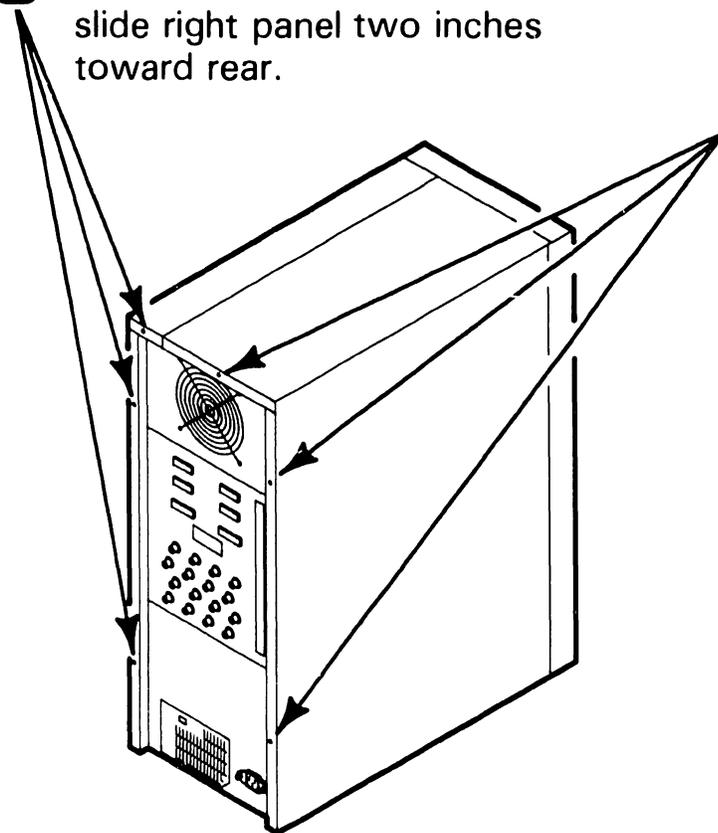
**3** Remove three screws and slide left panel two inches toward rear.
