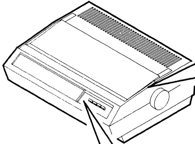
**1** Remove top cover by pressing locking tabs (inside) and lifting up.
