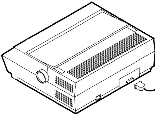
**3** Connect Master-to-Printer cable between printer and Master Unit. Tighten connector screws.
