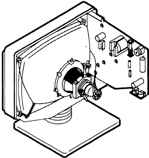
**8** Adjust horizontal width coil Z2 for a display width of  $8 \pm 1/8$  in. ( $20.3 \pm 3$  mm).
