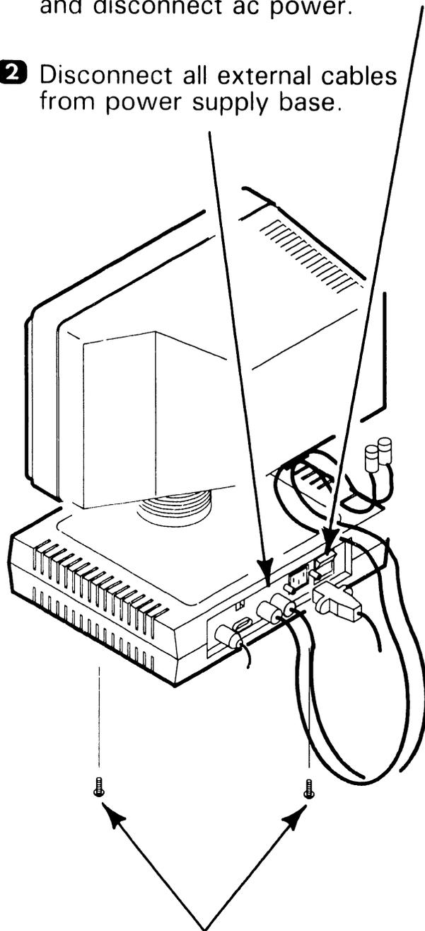
**3** Remove screws and monitor from power supply base.
