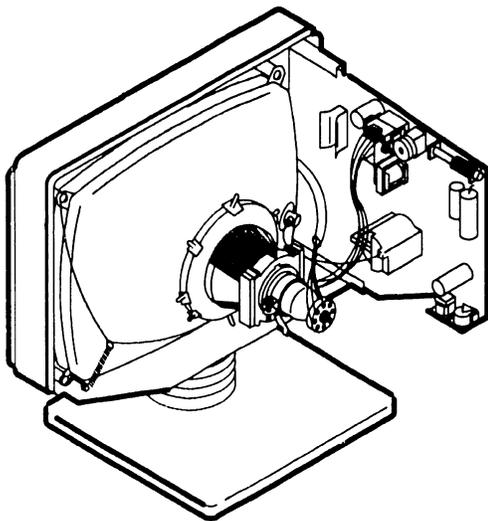
**5** Adjust vertical hold R6 to center of its stable range.
