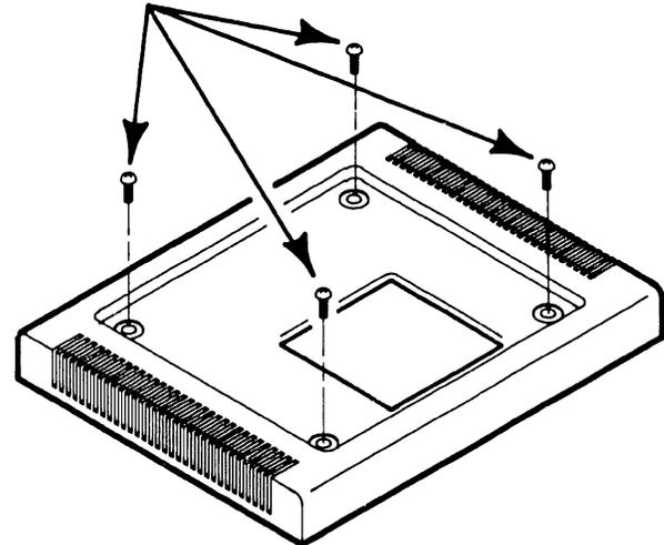
**5** Remove screw and pull switching power supply and rear panel from retaining tabs.
