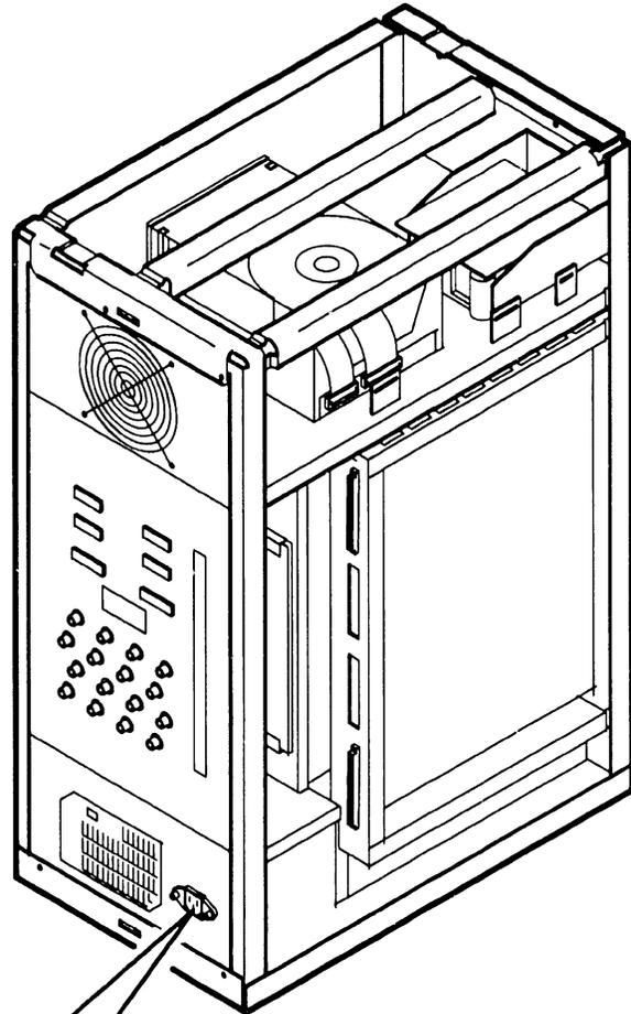
**7** Remove screws and filter.
