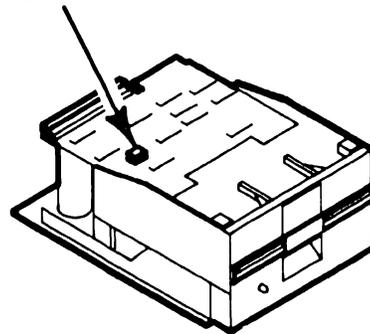
**6** For Tandon drive, adjust R4 until timing marks appear stationary.
