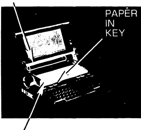
5 Load thermal paper into printer: hold down PAPER IN key to advance paper.
