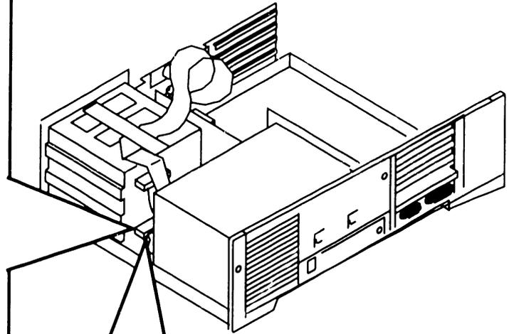
**7** Connect power supply cable and grounding strap to floppy drive "B".
