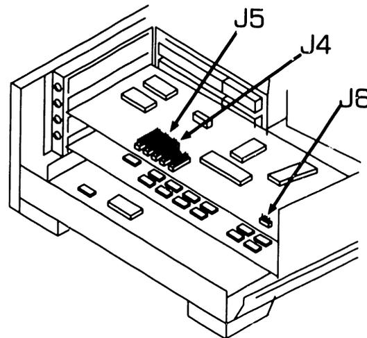
11 Connect hard disk select LED cable to J6 on the Winchester/Floppy Controller board.
