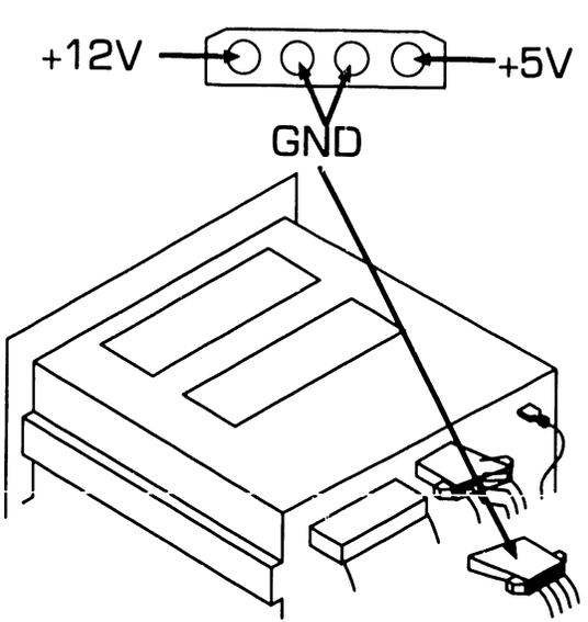
**4** Connect common lead of DVM to one of ground test points on floppy diskette power cable connector.
