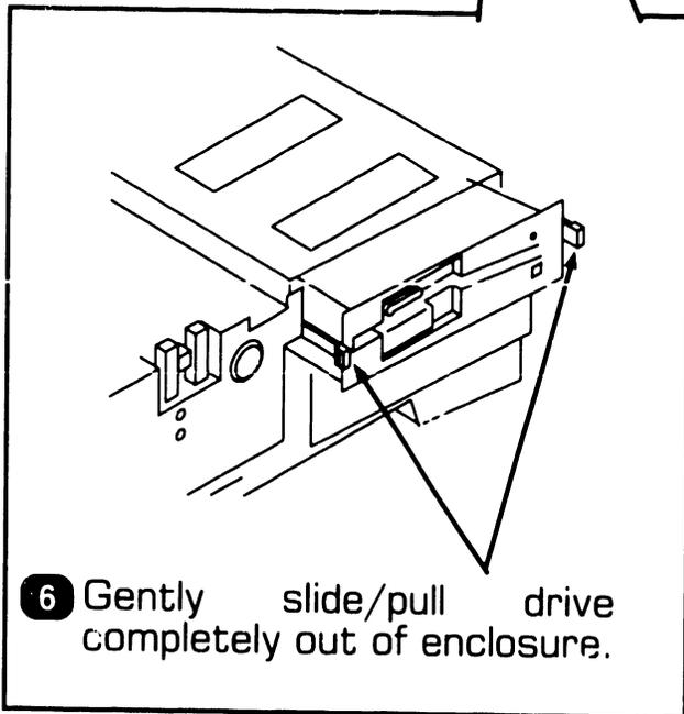
**6** Gently slide/pull drive completely out of enclosure.
