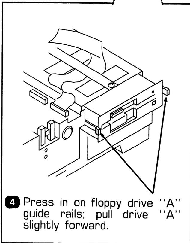
**4** Press in on floppy drive "A" guide rails; pull drive "A" slightly forward.
