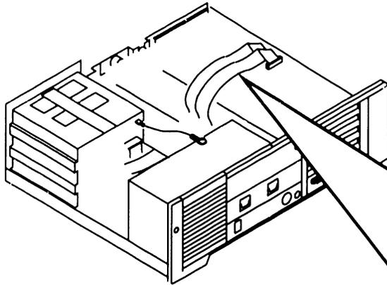
WINCHESTER/FLOPPY CONTROLLER BOARD CABLING CONNECTIONS:
