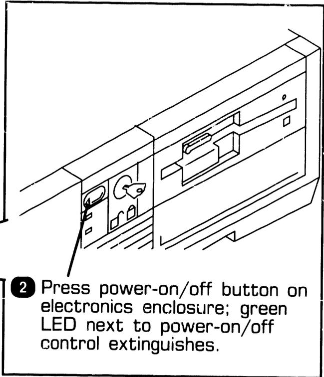
2 Press power-on/off button on electronics enclosure; green LED next to power-on/off control extinguishes.
