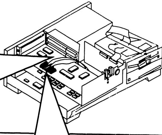
10 Connect drive "C" cables (220-3603 and 220-3604) to J4 and J5 on the Winchester/Floppy Controller board.
