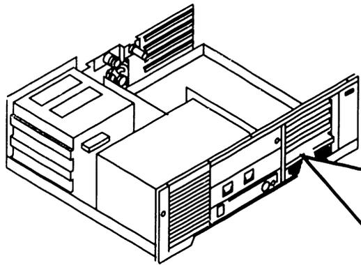
2 Remove synchronous/asynchronous board (➡7.2.3).
