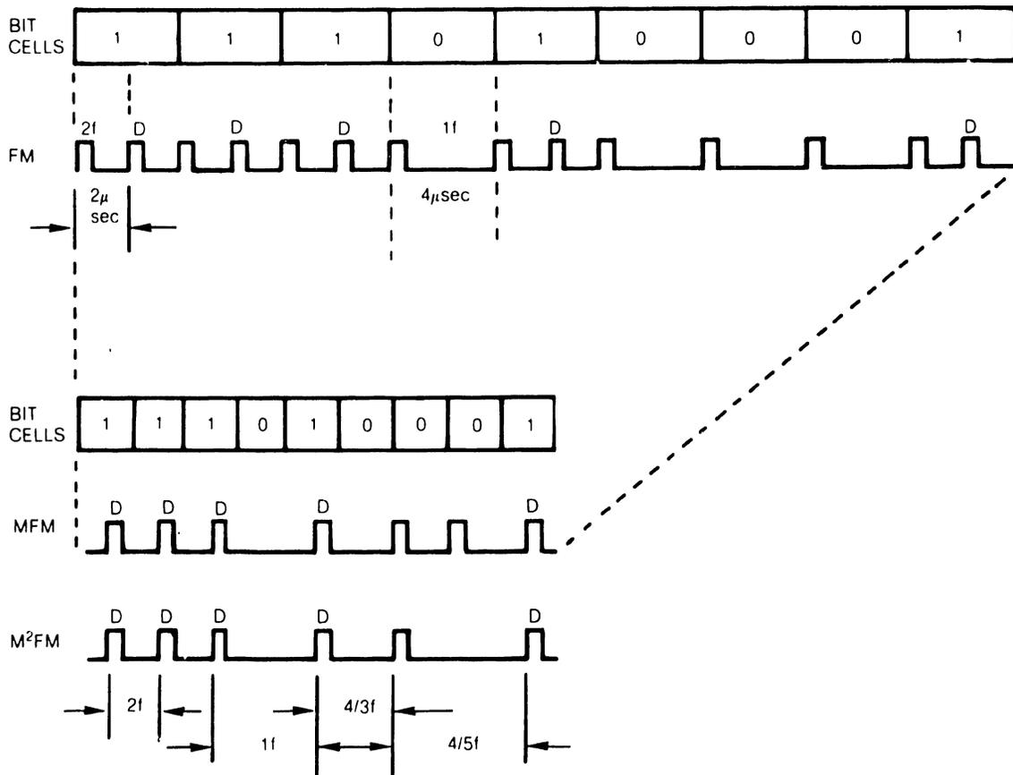
FIGURE 7. FM, MFM AND M<sup>2</sup>FM ENCODING
