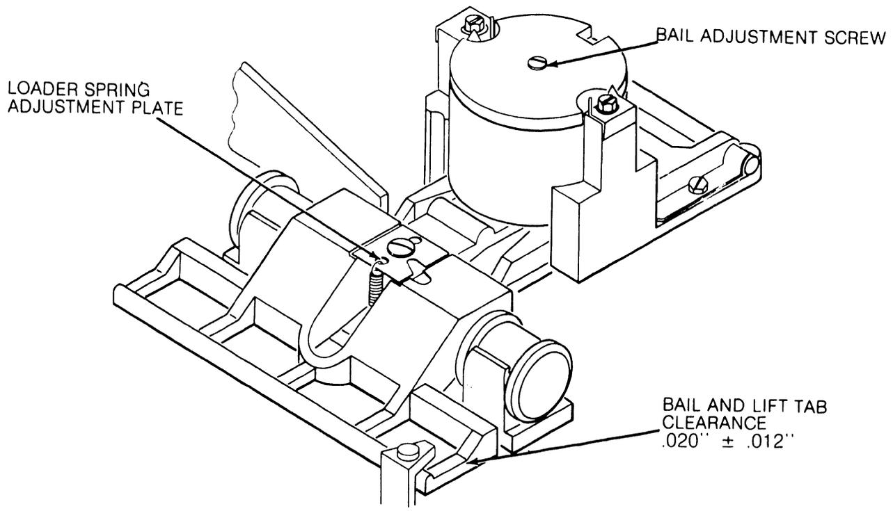
FIGURE 37. HEAD LOAD MECHANISM ADJUSTMENT
