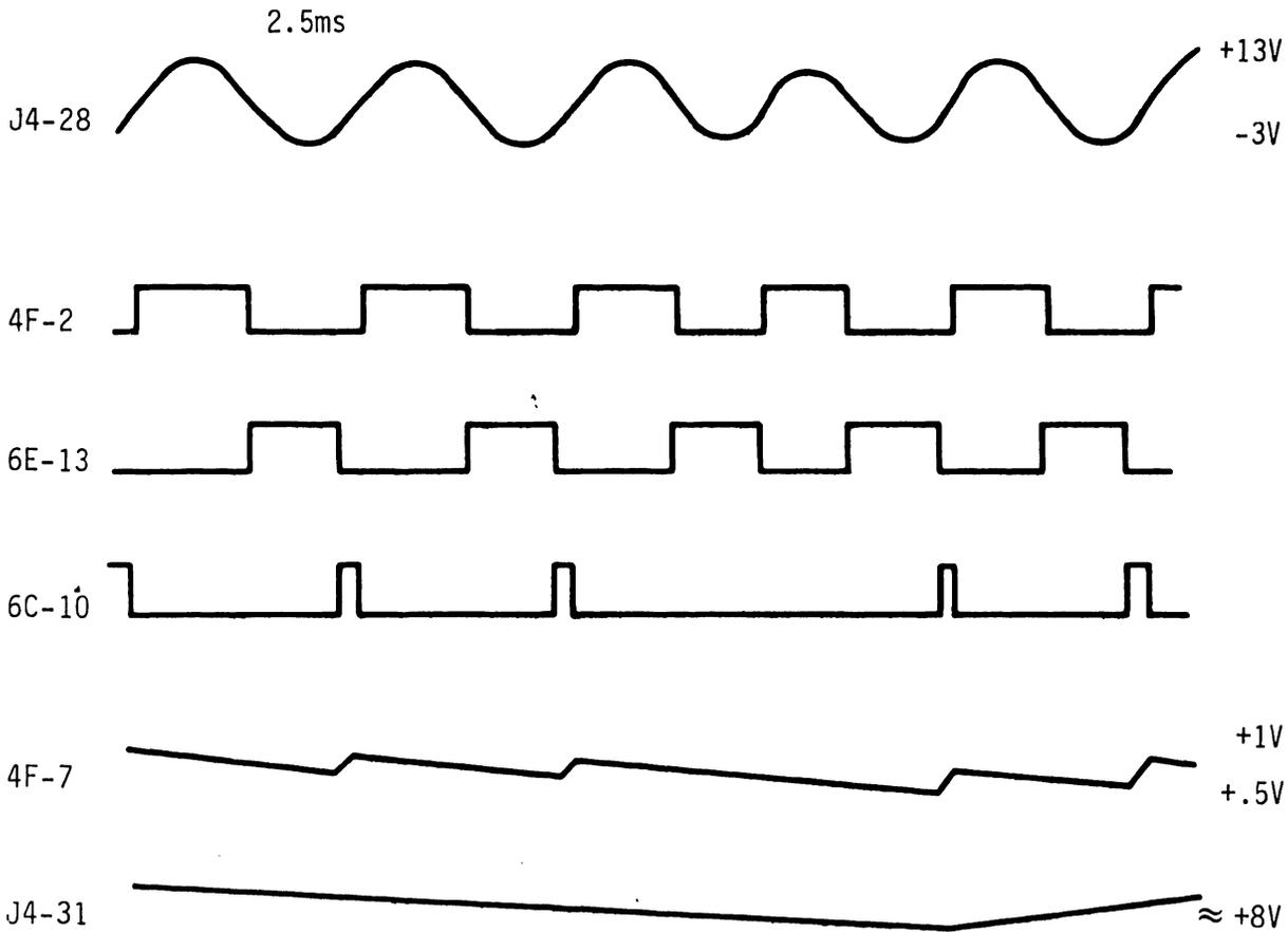
Figure 3-18: Motor Control Timing
