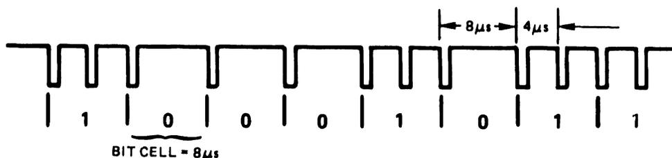
Figure 3-21: FM Encoding
