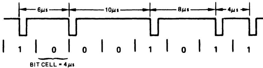
Figure 3-23: M<sup>2</sup>FM Encoding
