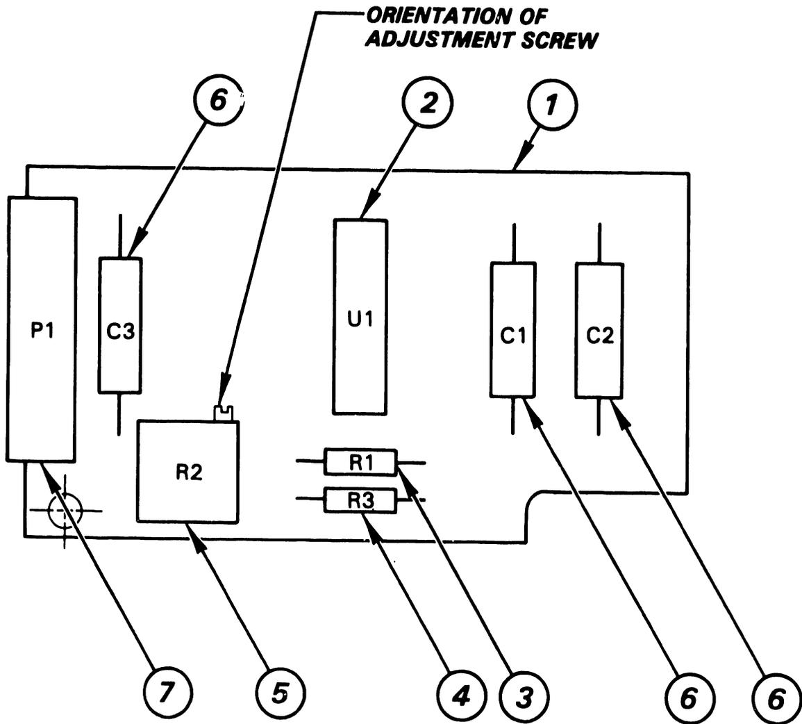
Figure B-3: Ready PCBA Component Layout
