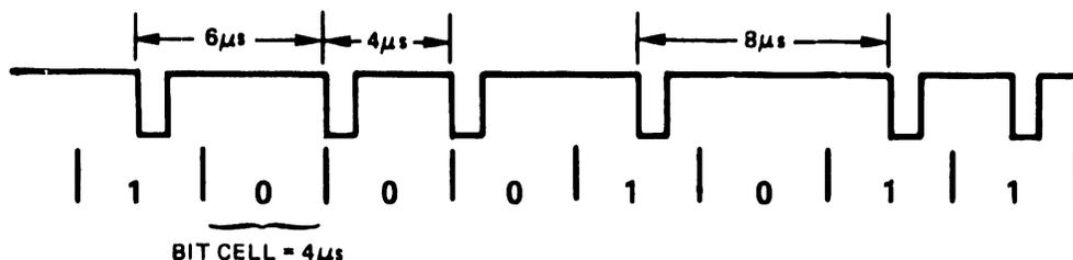
Figure 3-22: MFM Encoding
