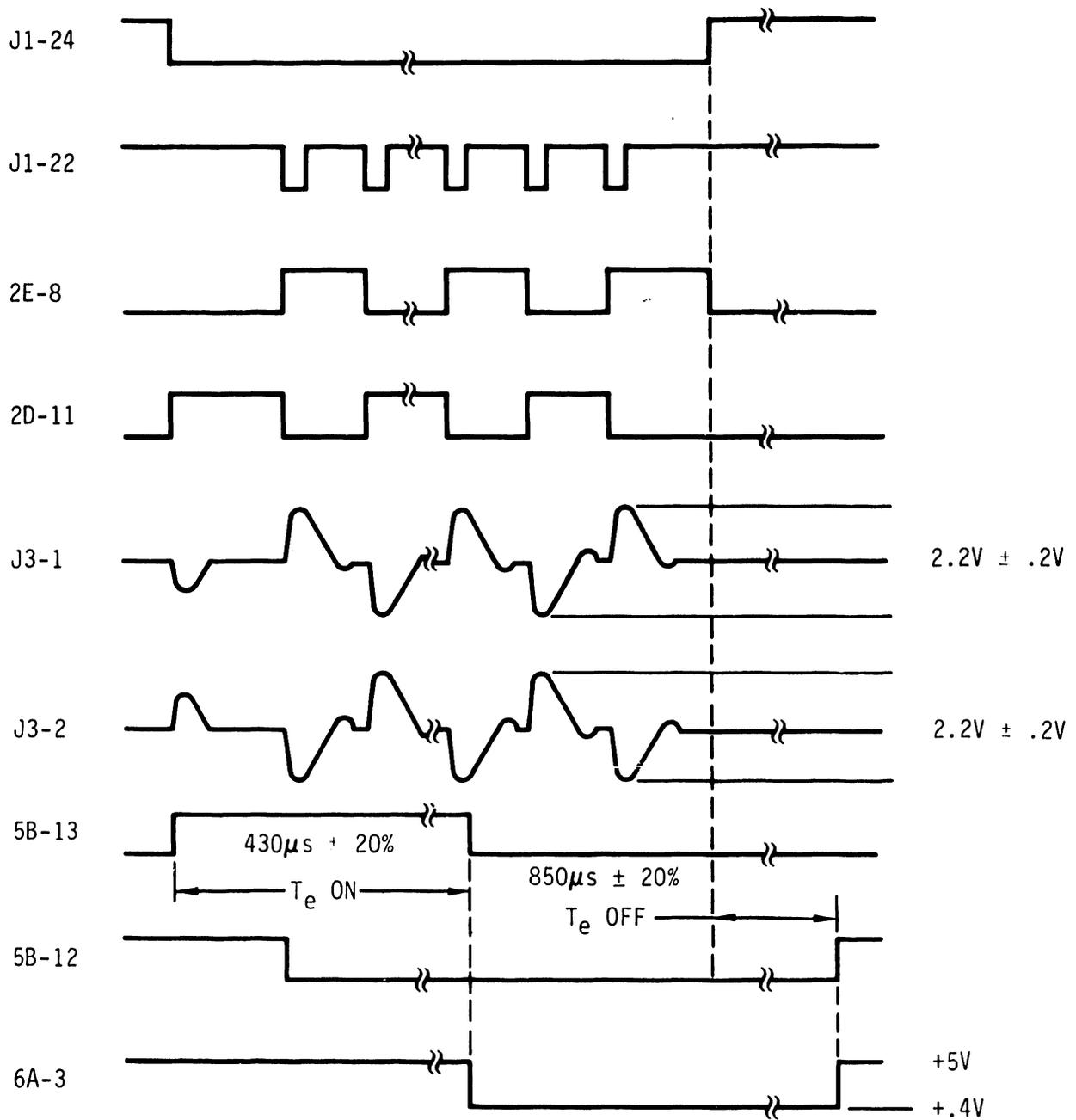
Figure 3-19: Write Timing
