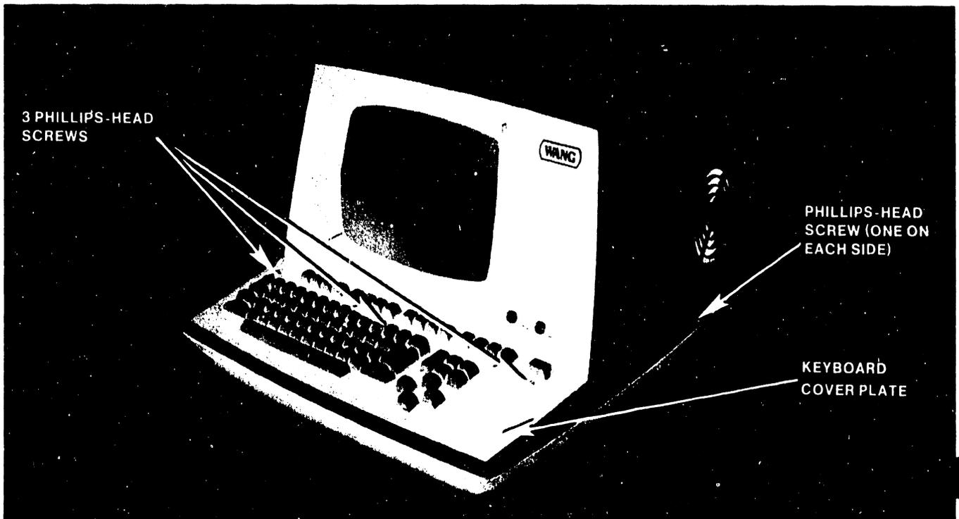
Figure 5-4. Cover Removal/Replacement
