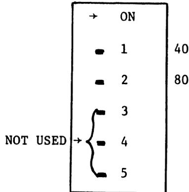
Set switches 1 and 2 OFF for a BOARD address of 01/05.
