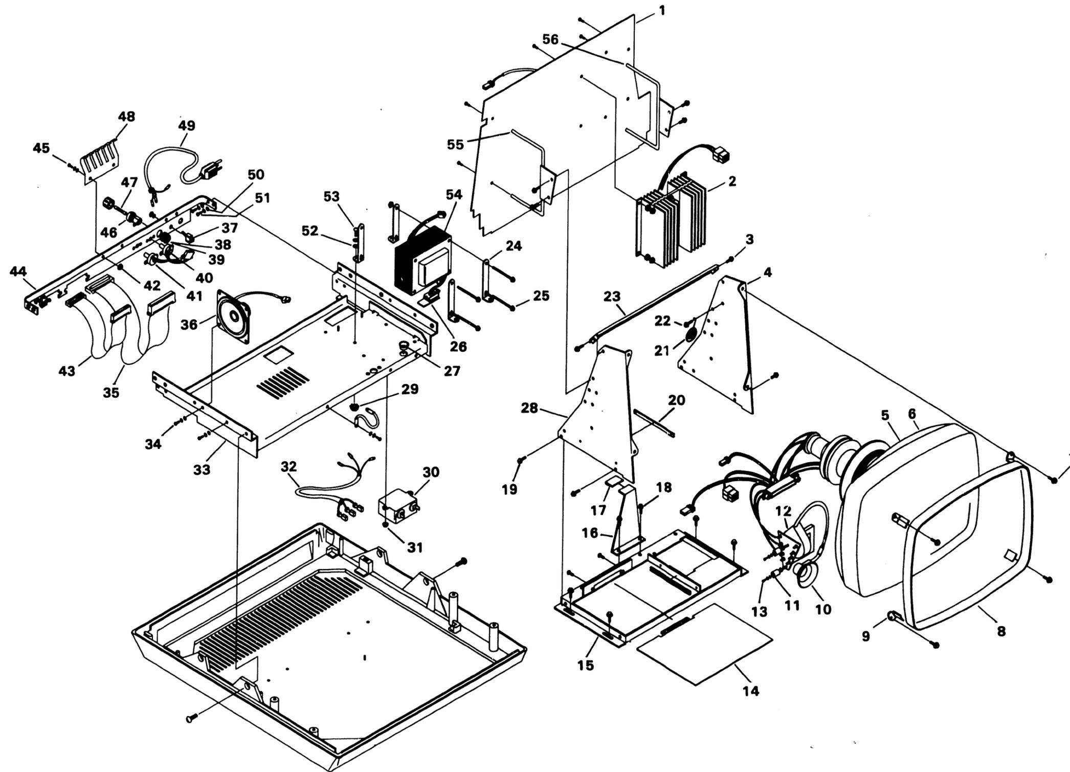
FIGURE 3 12" MONITOR & REAR PANEL ASSEMBLY
