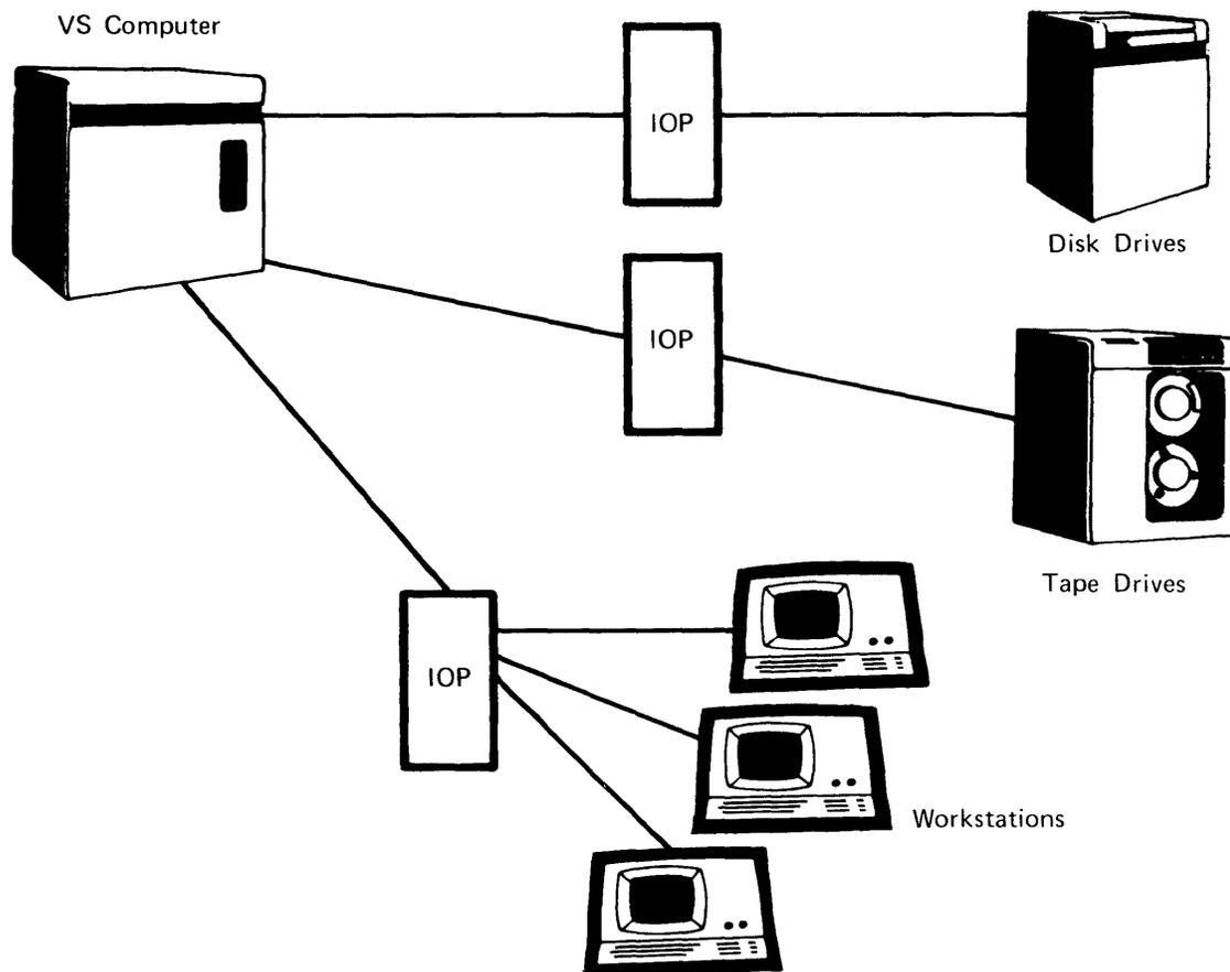
Figure 14. Diagram of VS Systems with IOPs
