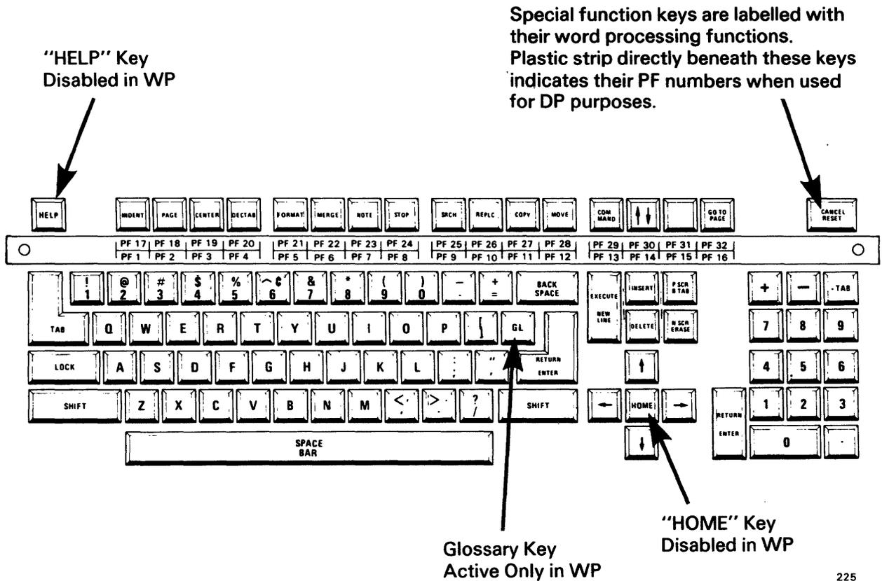
Figure 7. Keyboard of the 2246C Combined Workstation
