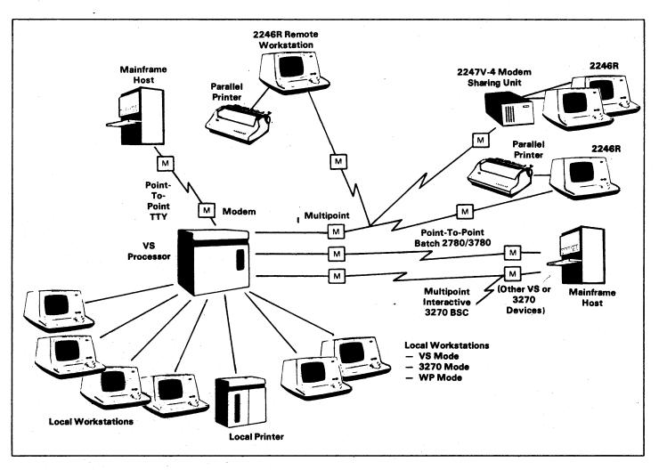
Wang VS Computer Systems can be configured with various data communications capabilities, including:
