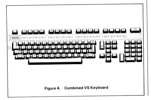
system-defined functions. In data processing mode, the PF keys are user-programmable. In word processing mode on combined workstations, these 16 keys provide word processing functions such as CENTER, SEARCH, and COPY. The red *HELP key* allows the user to interrupt processing and access other VS functions. It is disabled during word processing and at the option of the user.
