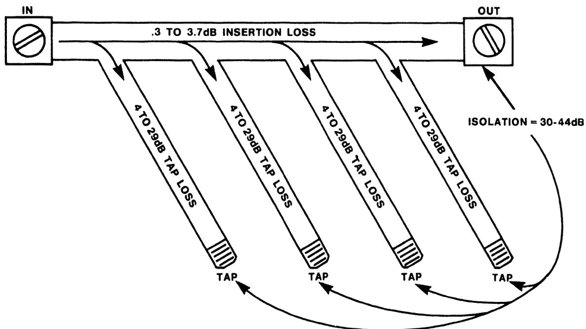
Figure 2-24 Directional Tap Functional Diagram
