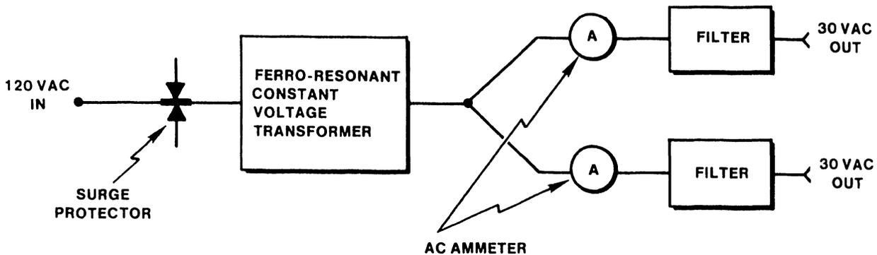
Figure 2-29 Power Converter Functional Diagram
