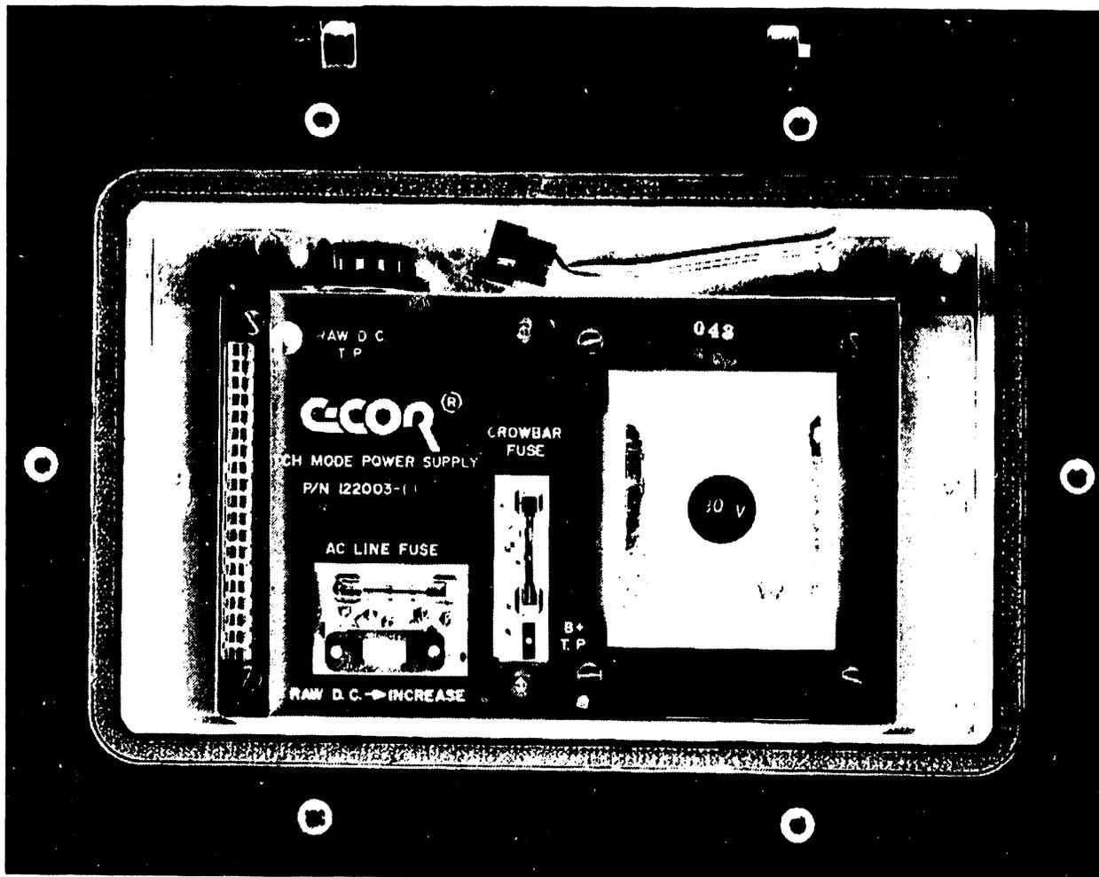
Figure 5-19 Diplexer Power Supply Module
