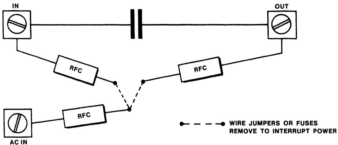
Figure 2-32 Power Combiner Functional Diagram
