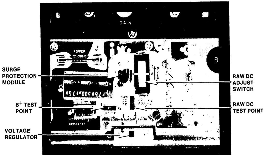
Figure 5-12 Amplifier Detail, Power Supply Area
