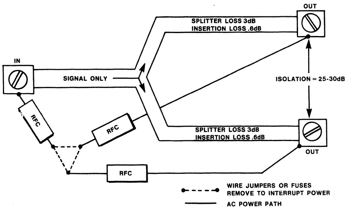
Figure 2-16 Splitter Functional Diagram
