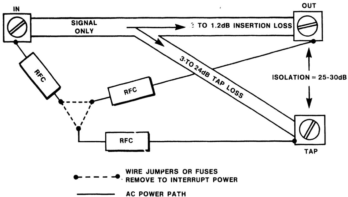
Figure 2-20 Directional Coupler Functional Diagram
