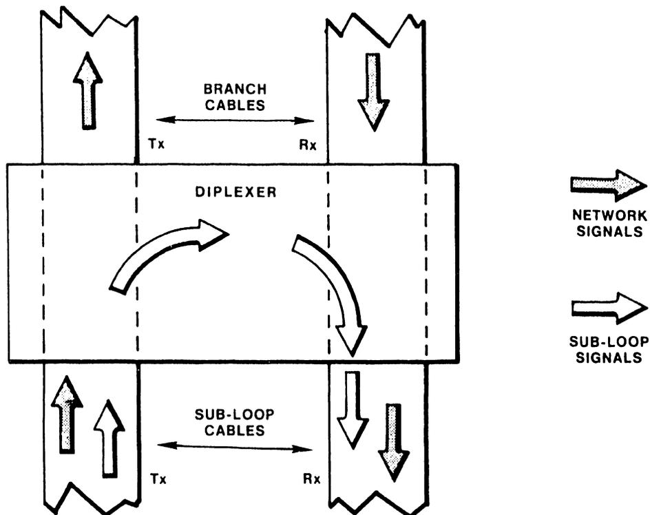
Figure 2-4 Diplexer Functional Diagram
