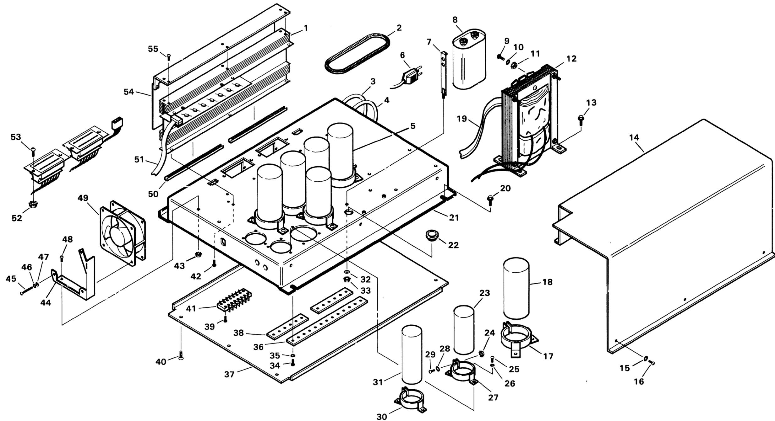
FIGURE 3 CHASSIS & TRANSFORMER ASSEMBLY
