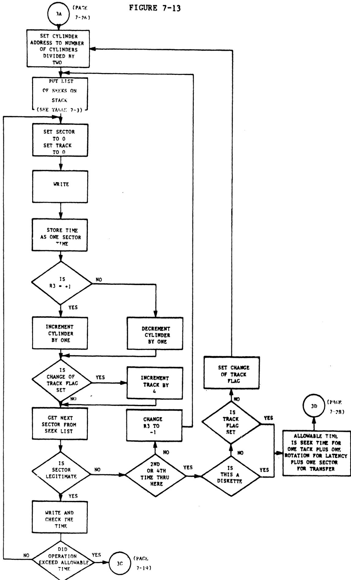
FLOWCHART 5B DISK TIMING TEST
