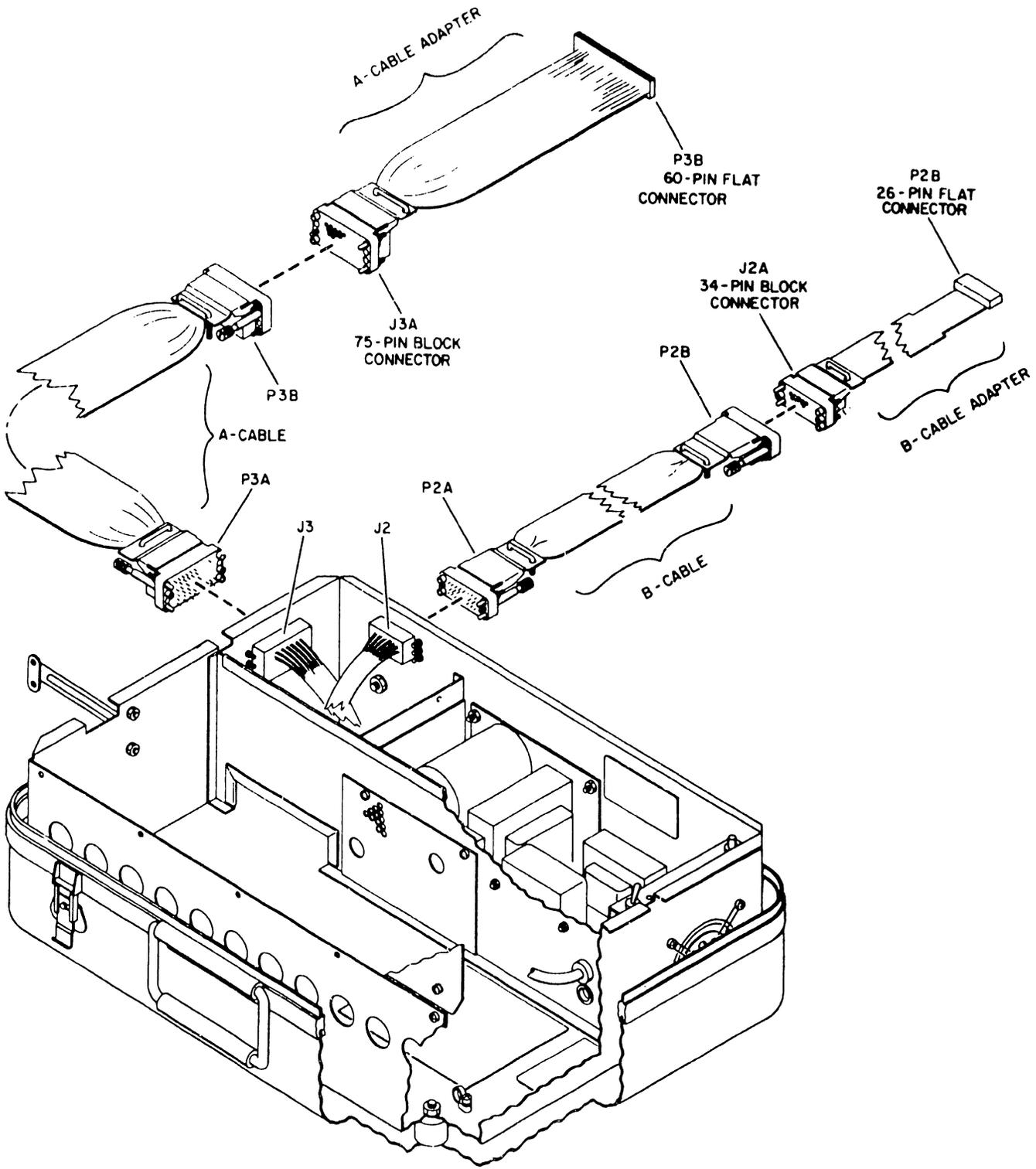
Figure 2-1. TB304A and Associated Hardware (Sheet 1)
