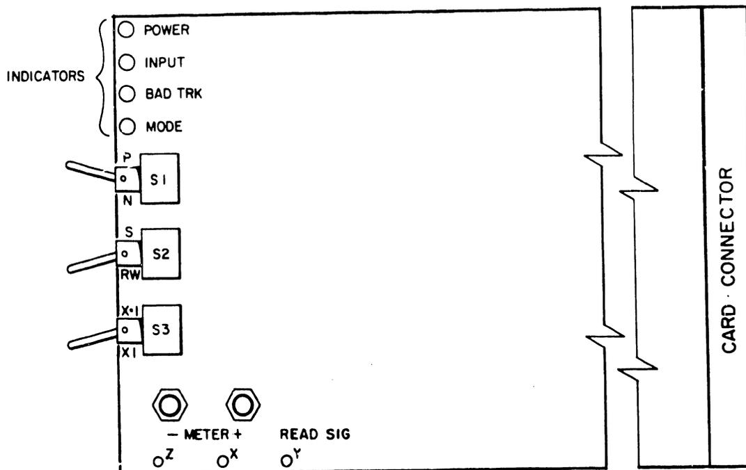
Figure 2-4. Head Alignment Card
