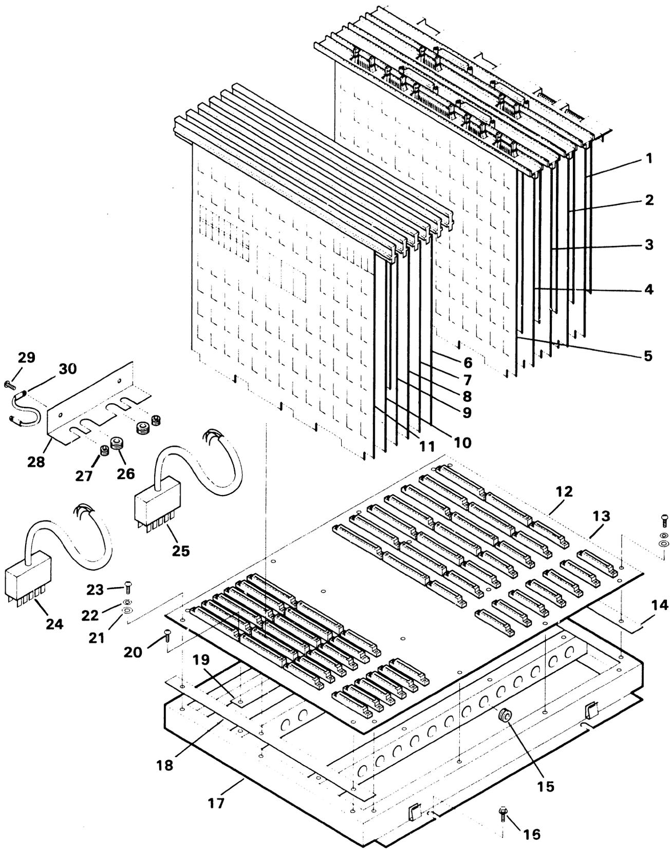
**FIGURE 4 2200 VS MOTHERBOARD ASSEMBLY
