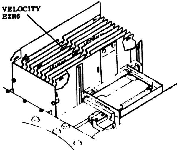
FIGURE 4-8 75 MEGABYTE VELOCITY GAIN ADJUSTMENT LOCATION
