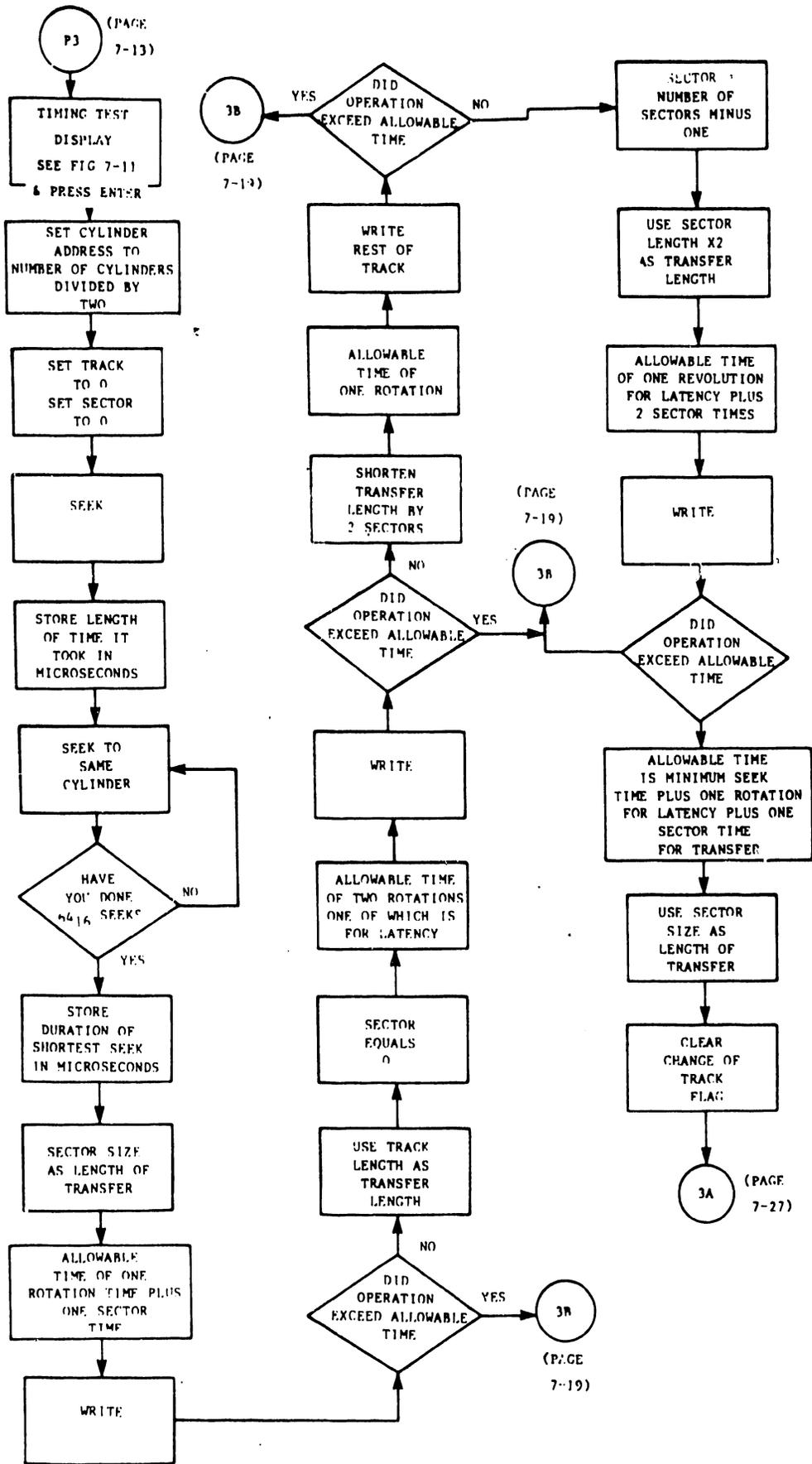
FLOWCHART 5A DISK TIMING TEST
