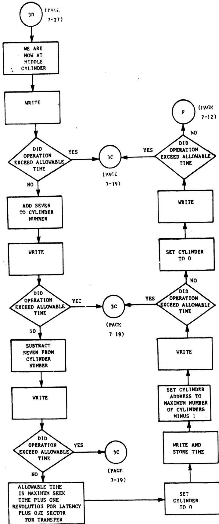
FLOWCHART 5C DISK TIMING TEST
