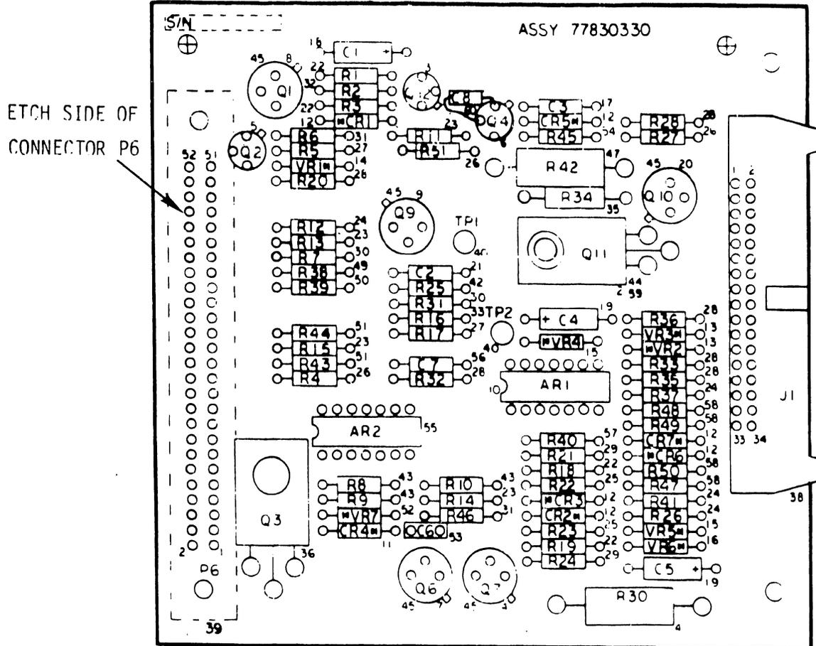
FIGURE 4-40 TOP VIEW OF POWER SUPPLY BOARD #2
