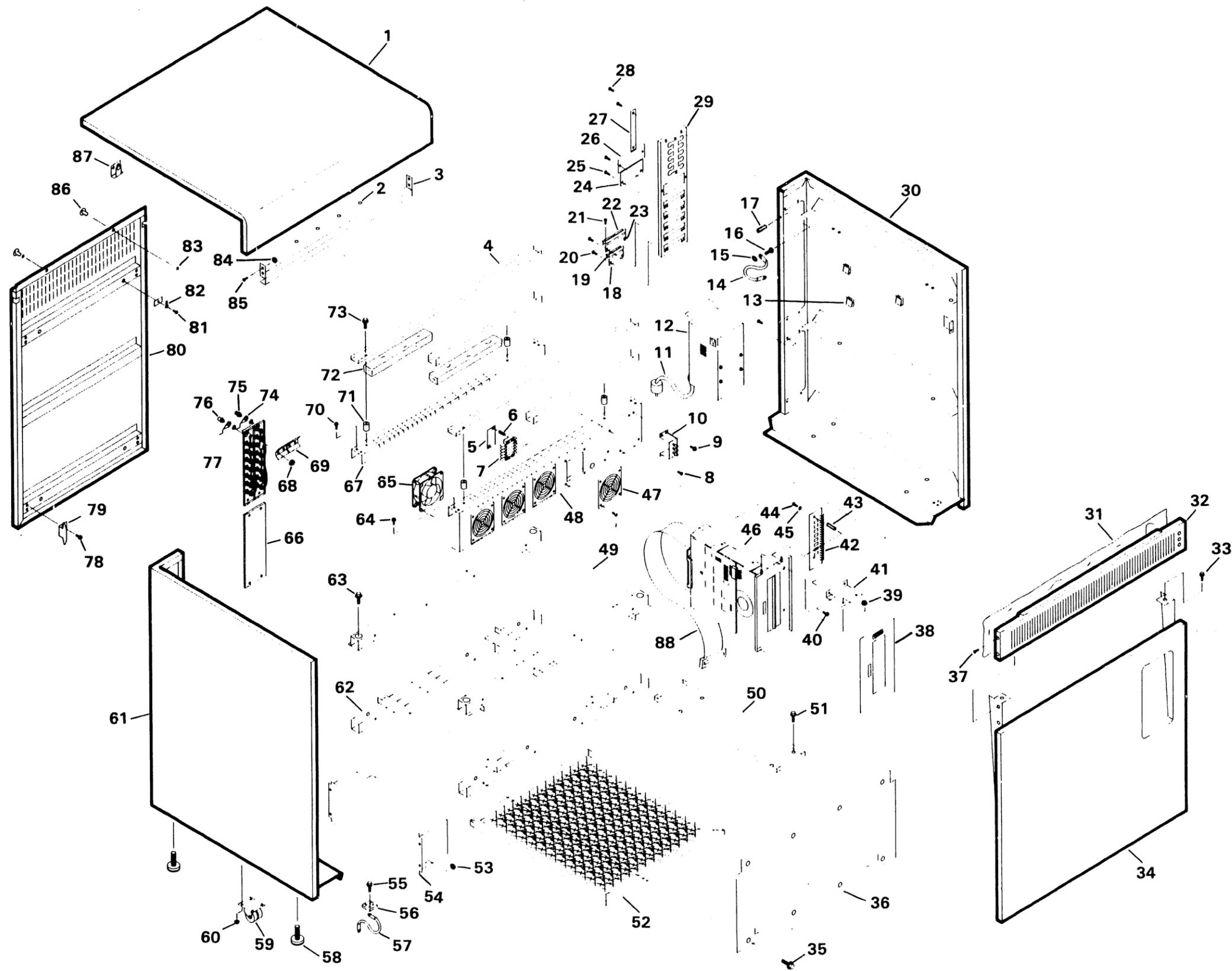
FIGURE 2 CABINET ASSEMBLY (ASSEMBLY PART NO. 279-4101)
