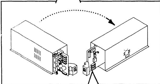
**13** Disconnect EAPA power cable from connector J7.
