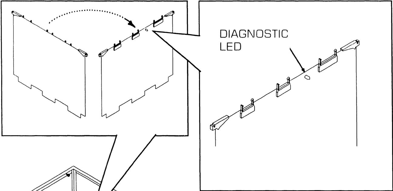
UISIO (Universal Intelligent Serial Input/Output) Controller runs PROM-based power-up diagnostics concurrently with the BP power-up diagnostics and completes in about ten seconds. The status of the UISIO diagnostics is indicated by a LED located at the upper center of the PCA. The LED will light during power-up diagnostics and then go out when the diagnostics have been completed successfully. If the LED stays on, the diagnostics have failed and the PCA may be defective.
