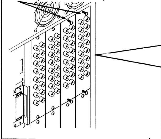
**8** Remove two mounting screws securing half-panel being removed.
