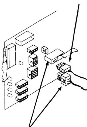
**14** Disconnect Motherboard power/signal cables from connectors J5 and J8.
