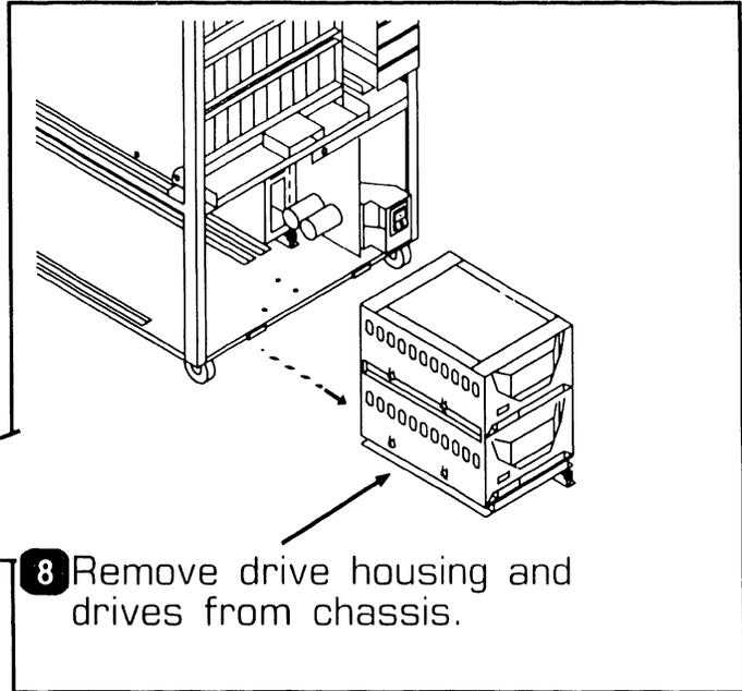
**8** Remove drive housing and drives from chassis.
