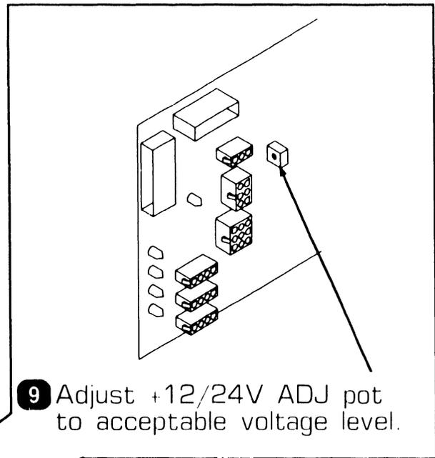
**9** Adjust +12/24V ADJ pot to acceptable voltage level.
