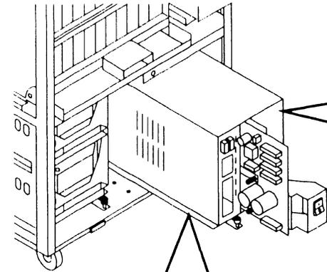
**15** Remove power supply from chassis.
