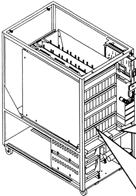
**7** Remove two Whiz-Loc screws securing card cage to chassis.
