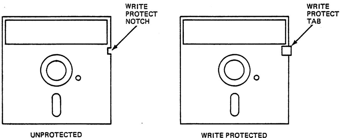
Figure 3-1. Write Protect Feature
