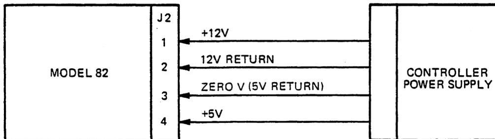
Figure 2-5. Interface Signals - Model 82
