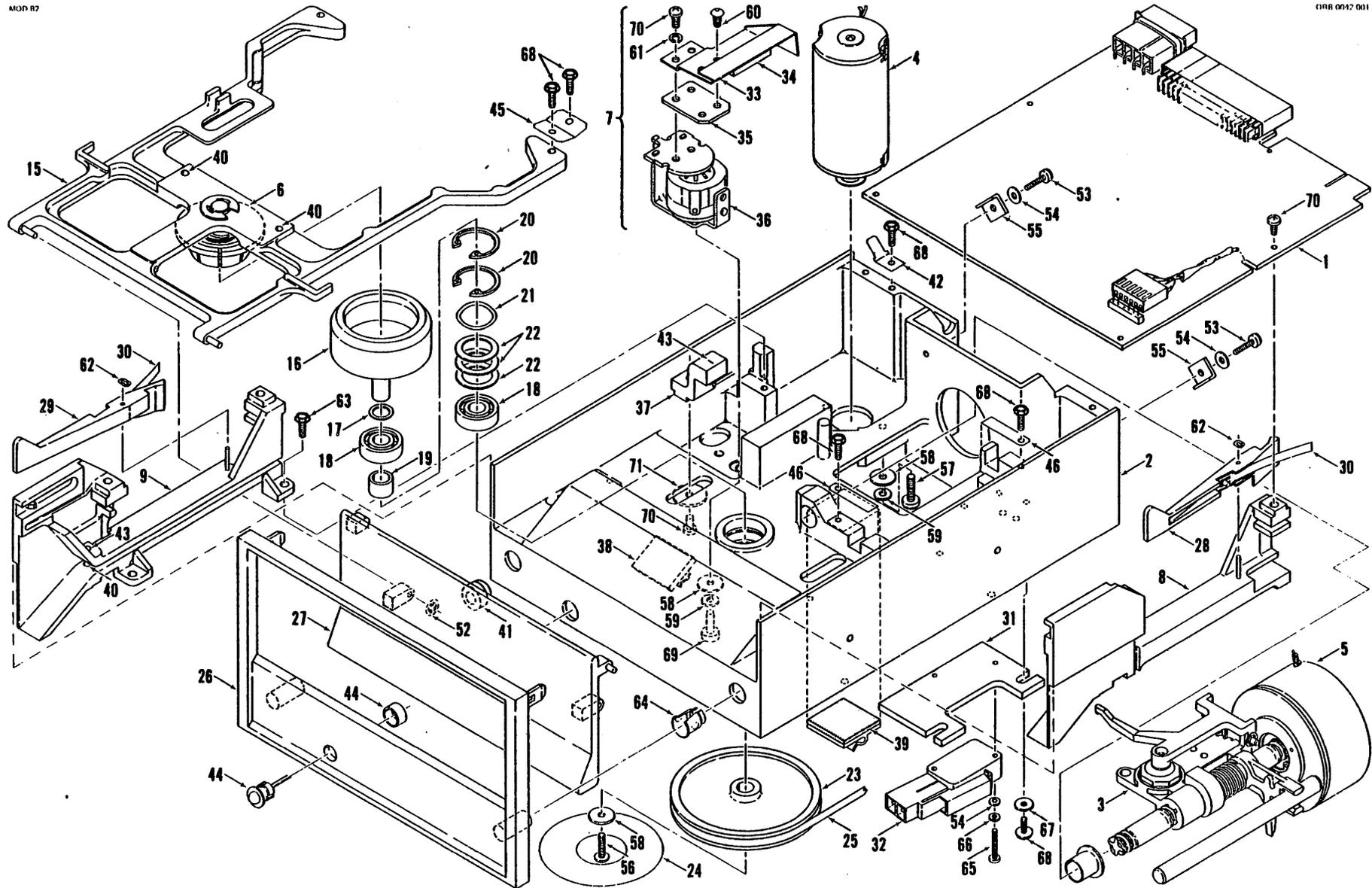
Figure D-1. Model R2 Microfloppy-Overall View
