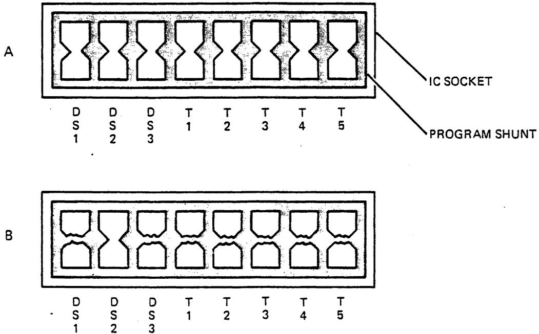
Figure 2-9. Program Shunt Module - Circuit Board 620311-001
