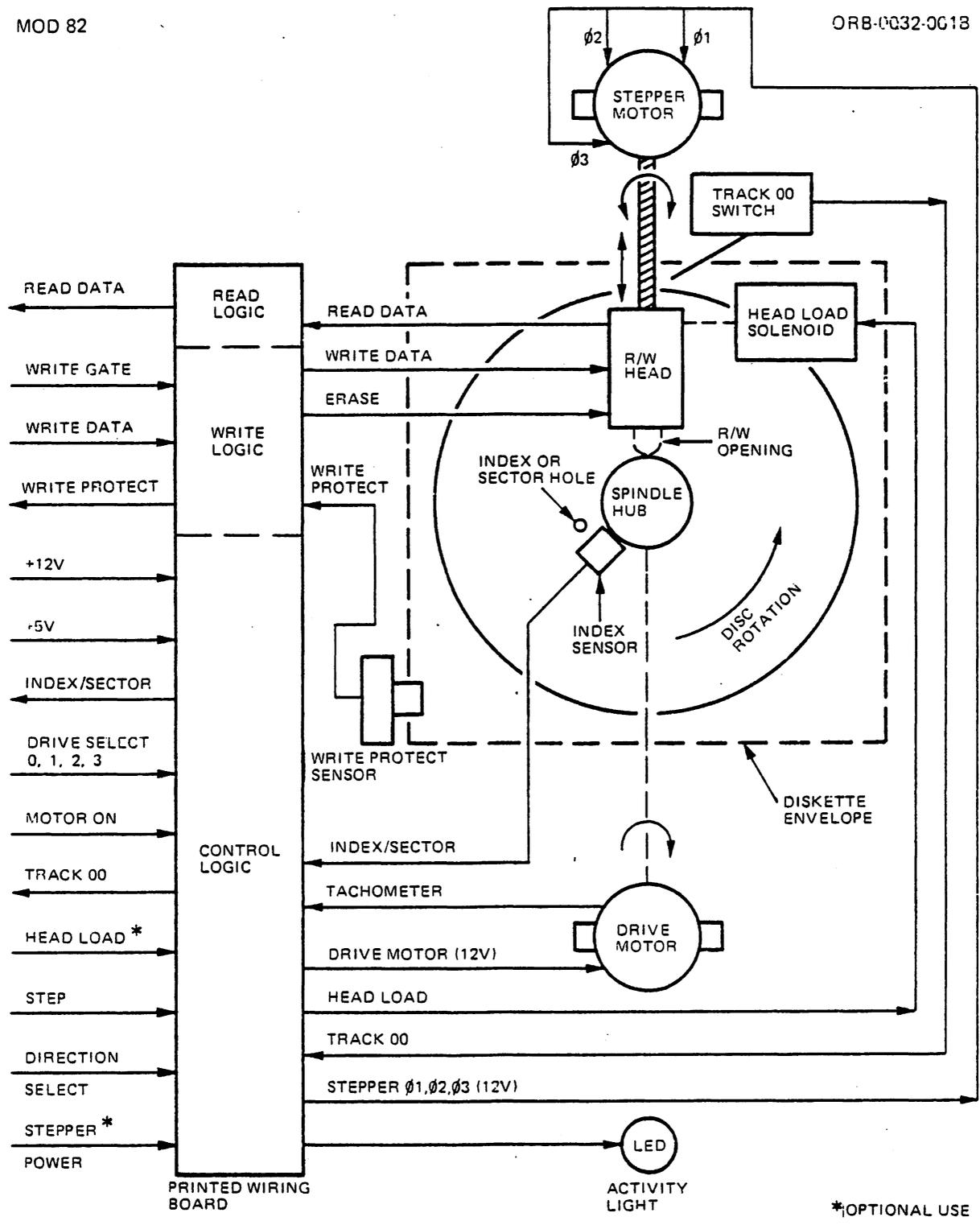
Figure 4-1. Functional Block Diagram
