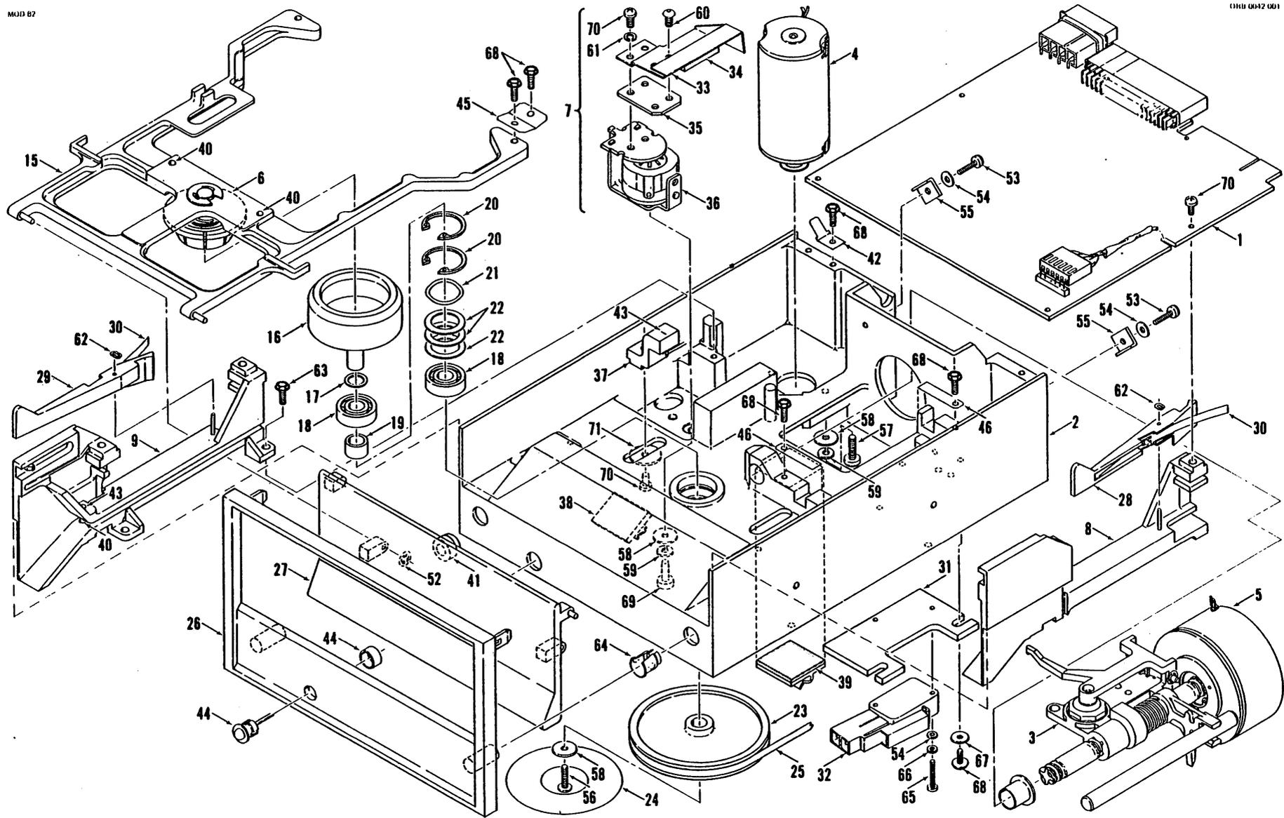
Figure D-1. Model 82 Microfloppy-Overall View
