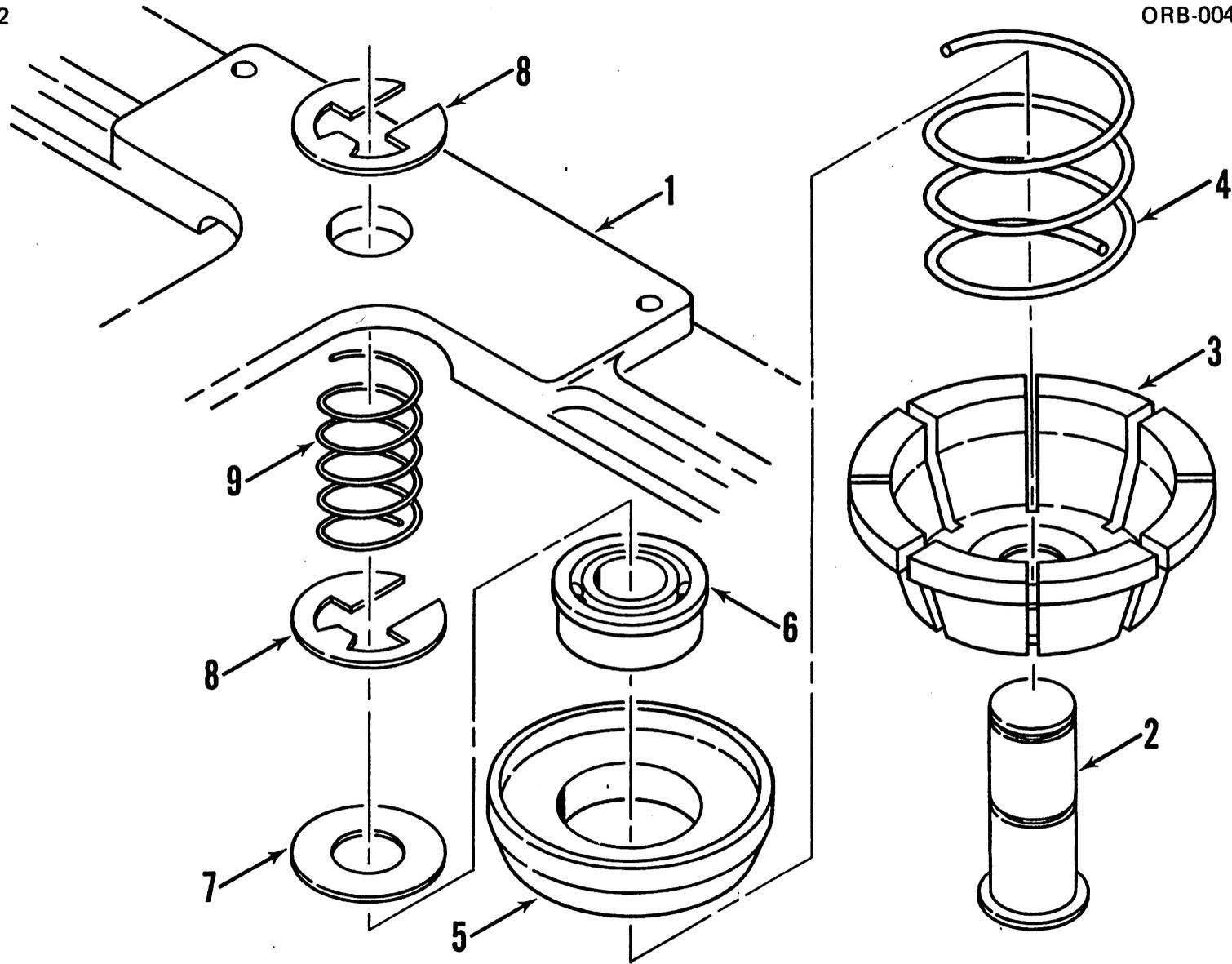
Figure D-2 Model 82 Microfloppy - Carrier Assembly
