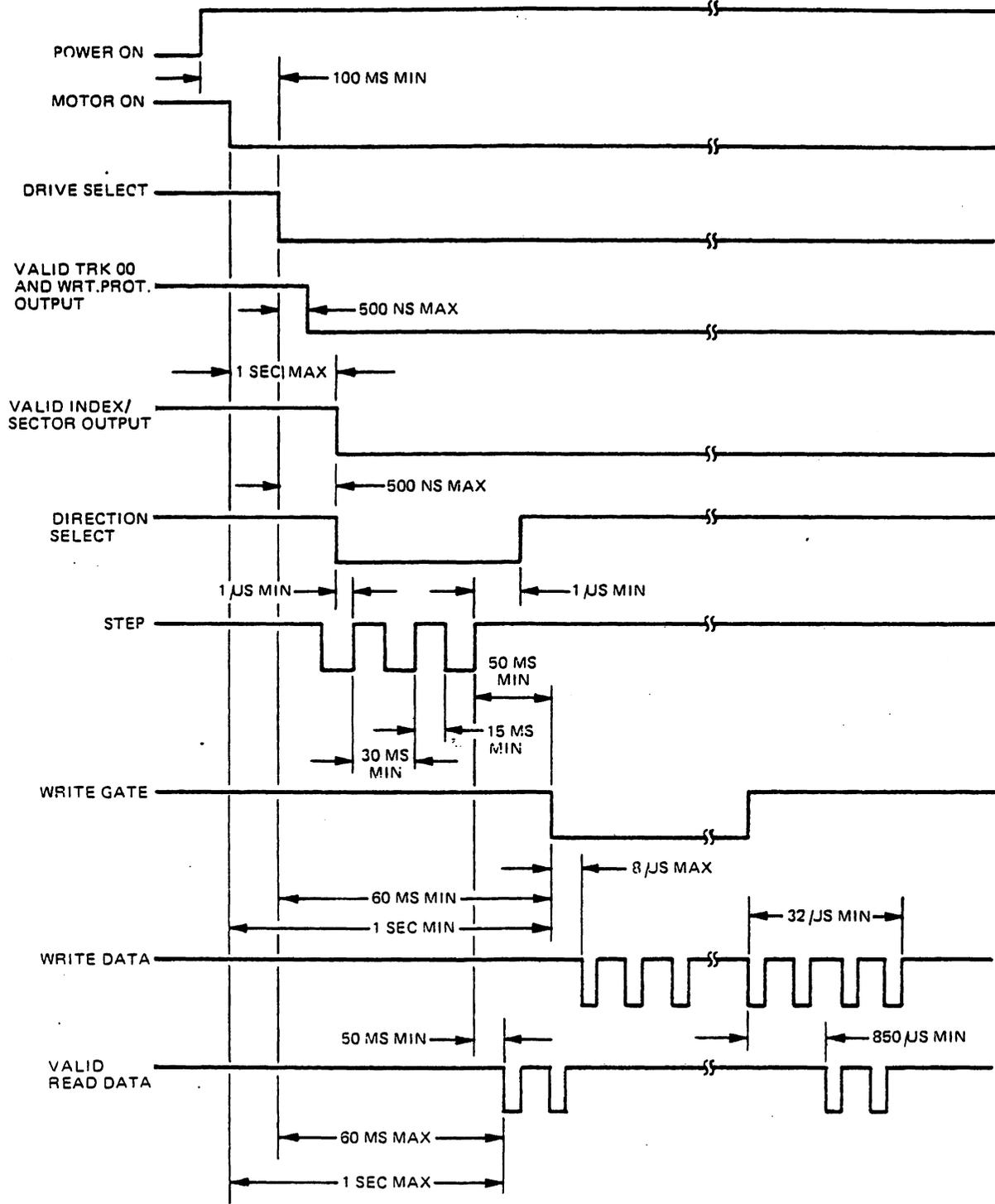
Figure 2-6. Model 82 Interface Timing Requirements
