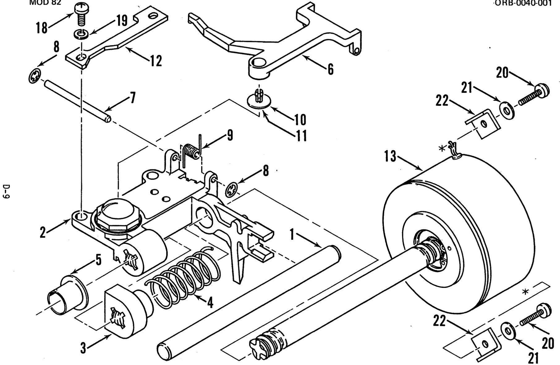
Figure D-3 Model 82 Microfloppy - Carriage Assembly
