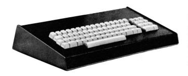
KEYBOARD The keyboard is a delight to use. The main keys are arranged and sculptured to be the same as a standard Selectric typewriter, making it easy to switch between keyboards. In addition to the Selectric keys are the keys required to generate the upper/lower case ASCII character set. A 10 key calculator entry pad is also provided for numeric data entry. The keyboard has the feel of a Selectric, but has no contacts in the switches. It is done electronically for reliability.
