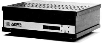
JUPITER III AT The Jupiter III AT mainframe is a table top version utilizing the Z80 processor on the CPU card.
