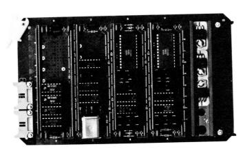
SPI-027 The Serial/Parallel Interface has one RS-232-C serial interface as in the DSD-125, and two independent eight bit parallel data channels as in the DPD-125. One quarter of the card is spare for custom interfaces to be added. Cables must be ordered separately.
