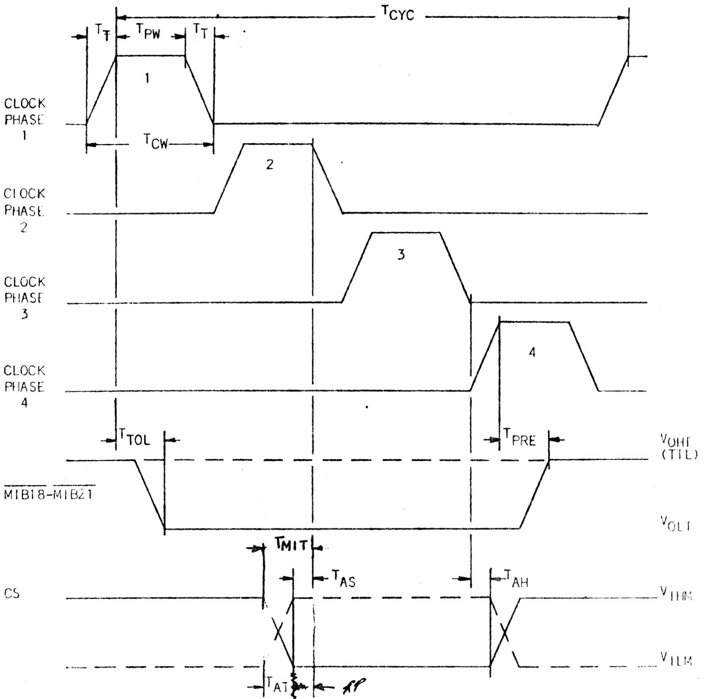
NOTE: TTL outputs (MIB18-MIB21) are unconditionally driven high at  $\emptyset 4$  and conditionally driven low at  $\emptyset 1$ . This conditional low will be valid until the next  $\emptyset 4$ .
