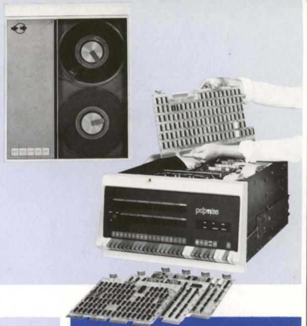
The Western Peripherals TC-130 Magnetic Tape Controller offers users the convenience of both Phase Encoded and NRZ formats consolidated onto plug-in PC boards. In addition, it provides the ability to mix 7-track and 9-track NRZ, PE or dual-density tape units in any combination up to eight units.
