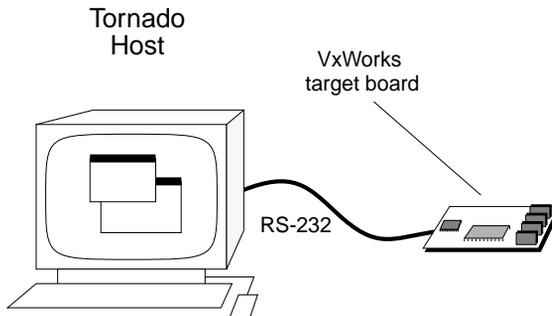
Figure 2-1 illustrates a minimal cross-development configuration: the target is a bare board, connected to the host development system by a single serial line. When you connect the host and target exclusively over serial lines, you must:
