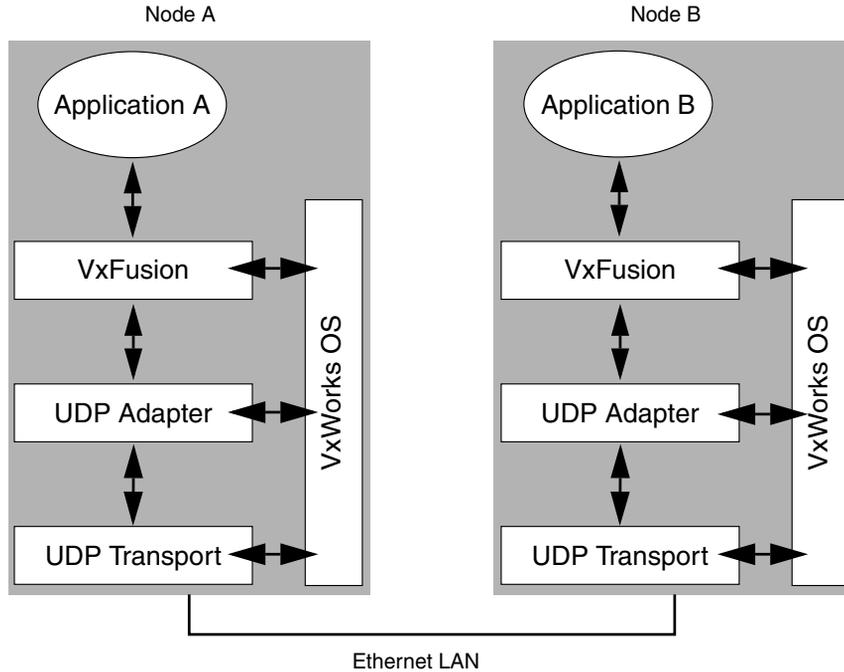
Figure 10-1 illustrates an example two-node VxFusion system. VxFusion has been installed on each of the two nodes that are connected to the same subnet of an Ethernet LAN. Because the two nodes are connected by Ethernet, TCP, UDP, IP, and raw Ethernet are all possible transports for communications.
