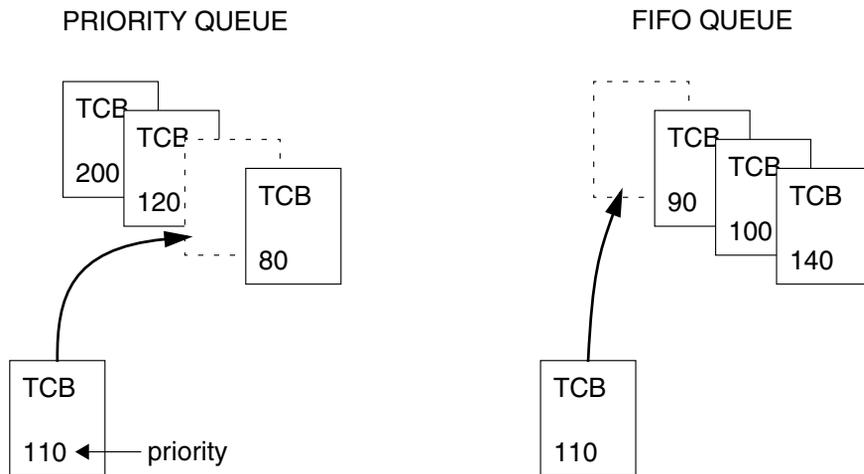
Priority ordering better preserves the intended priority structure of the system at the expense of some overhead in `semTake()` in sorting the tasks by priority. A FIFO queue requires no priority sorting overhead and leads to constant-time performance. The selection of queue type is specified during semaphore creation with `semBCreate()`, `semMCreate()`, or `semCCreate()`. Semaphores using the priority inheritance option (`SEM_INVERSION_SAFE`) must select priority-order queuing.
