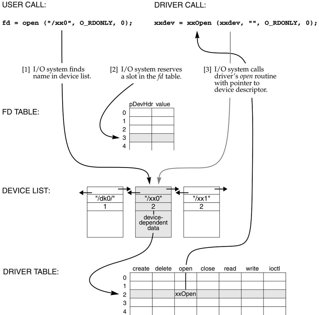
Again, the value entered in the *fd* object has meaning only for the driver, and is arbitrary as far as the I/O system is concerned.
