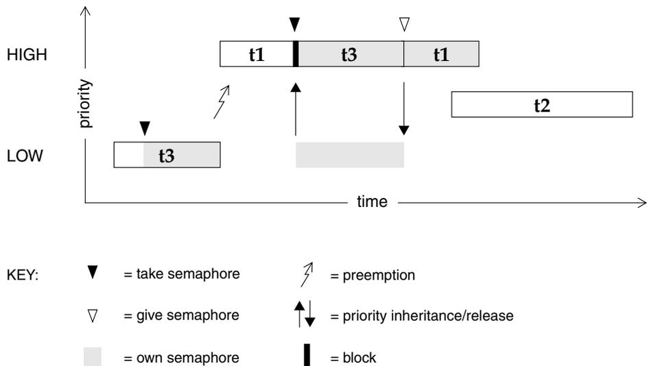
In Figure 2-12, priority inheritance solves the problem of priority inversion by elevating the priority of **t3** to the priority of **t1** during the time **t1** is blocked on the semaphore. This protects **t3**, and indirectly **t1**, from preemption by **t2**.
