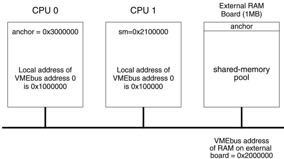
In the example configuration in Figure 11-5, the shared memory is on a separate memory board. On the Params tab for the master, `SM_OFF_BOARD` is TRUE, `SM_ANCHOR_ADRS` is 0x3000000, `SM_OBJ_MEM_ADRS` is set to `SM_ANCHOR_ADRS`, and `SM_OBJ_MEM_SIZE` is set to 0x100000. For the slave board, `SM_OFF_BOARD` is TRUE and the anchor address is 0x2100000. This is calculated by taking the VMEbus address of the memory board (0x2000000) and adding it to the local VMEbus address (0x100000).
