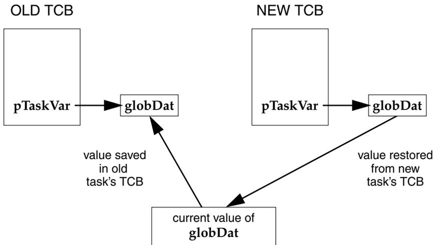
Use this mechanism sparingly. Each task variable adds a few microseconds to the context switching time for its task, because the value of the variable must be saved and restored as part of the task's context. Consider collecting all of a module's task variables into a single dynamically allocated structure, and then making all accesses to that structure indirectly through a single pointer. This pointer can then be the task variable for all tasks using that module.
