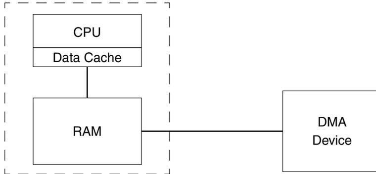
If a CPU writes data to RAM that is destined for a DMA device, the data can first be written to the data cache. When the DMA device transfers the data from RAM, there is no guarantee that the data in RAM was updated with the data in the cache. Thus, the data output to the device may not be the most recent—the new data may still be sitting in the cache. This data incoherence can be solved by making sure the data cache is flushed to RAM before the data is transferred to the DMA device.
