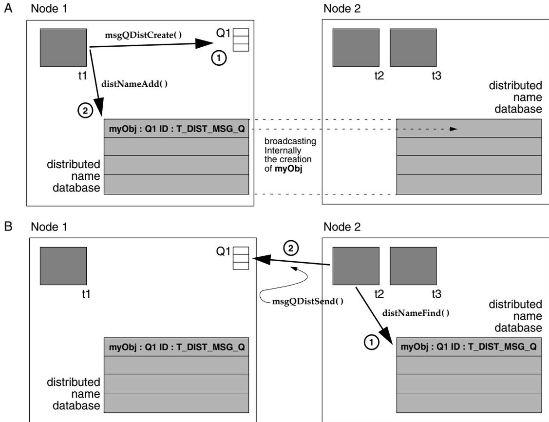
Task **t1** on Node 1 creates a message queue. The distributed message queue ID is returned by the creation routine. Task **t1** adds the ID and its associated name, **myObj**, to the distributed name database. This database entry is then *broadcast* to all nodes in the system. For task **t2** on Node 2 to send a message to this distributed
