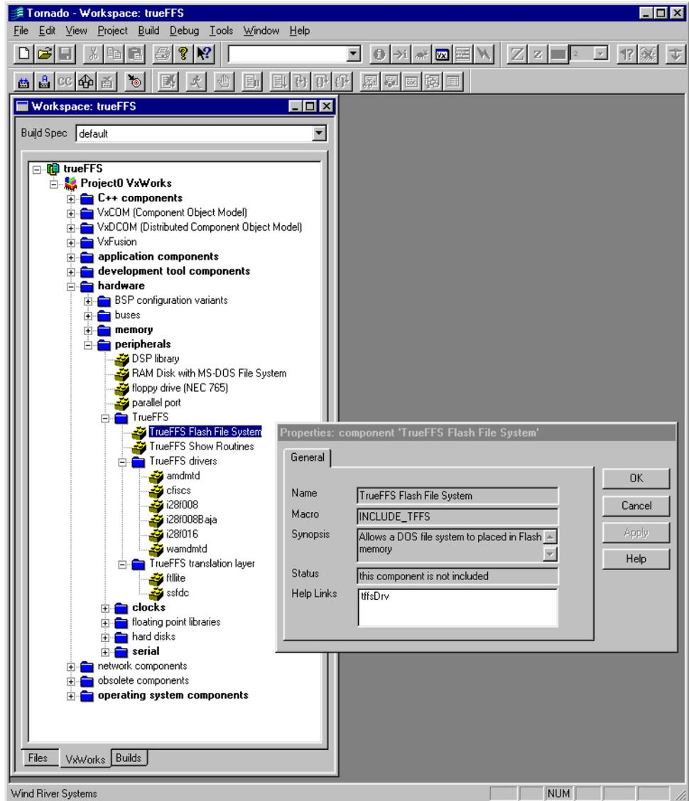
Defining this component triggers the correct sequence of events, at boot time, for initializing this product. It also ensures that the socket driver is included in your project (see 8.5.6 *Adding the Socket Driver*, p.305).
