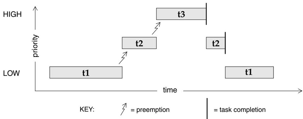
The disadvantage of this scheduling algorithm is that, when multiple tasks of equal priority must share the processor, if a single task is never blocked, it can usurp the processor. Thus, other equal-priority tasks are never given a chance to run. Round-robin scheduling solves this problem.
