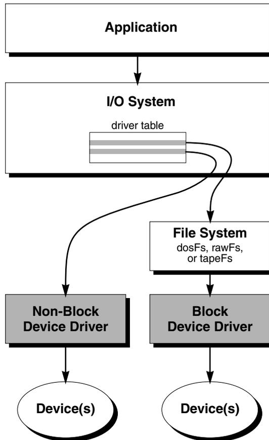
After a device is initialized for use with a particular file system, all I/O operations for the device are routed through that file system. To perform specific device operations, the file system in turn calls the routines in the specified **BLK\_DEV** or **SEQ\_DEV** structure.
