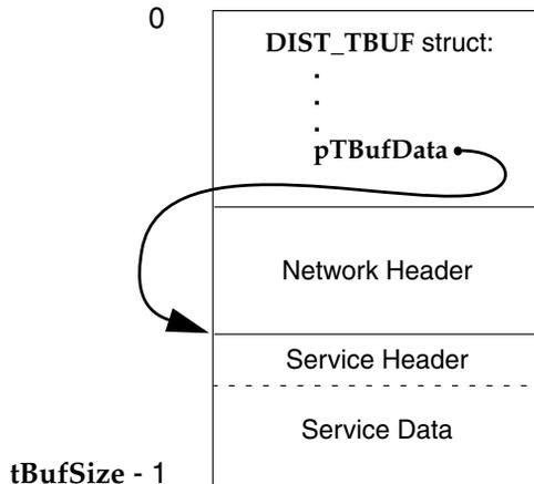
The `DIST_TBUF` structure member, `pTBufData`, contains the address of the start of the service header. To access the network header, subtract the size of the network header from this address.
