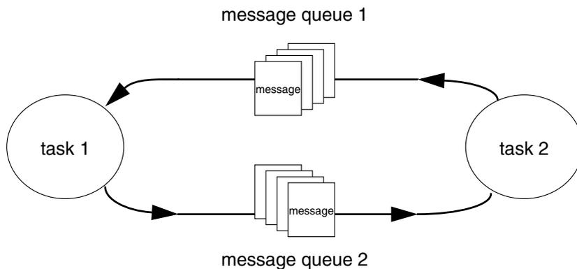
Multiple tasks can send to and receive from the same message queue. Full-duplex communication between two tasks generally requires two message queues, one for each direction; see Figure 2-14.
