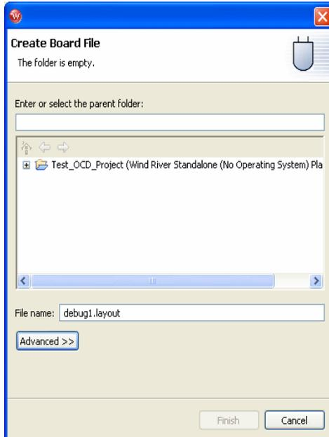
Wind River Workbench automatically populates the **Parent Folder** field with your active project. In the **File Name** field, type a name for your board file. This creates a **.layout** file, which JTAG Editor will use to create a **.brd** file in the next step.
