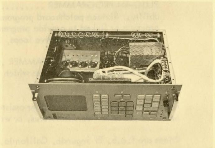
The Model KD-01 Keyboard Display unit provides the Arithmetic Processor with all the manual operation capability of the Wyle Scientific. It enables manual data entry and control of computation and provides a continuous visual display of all contents of all registers. It is a separate rack mounted unit which does not interfere with any of the operations previously described.
