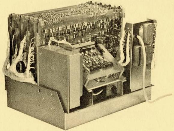
The Wyle Arithmetic Processor, Model AP-01, is an electronic unit which provides the full range of arithmetic operations in an unusually simple and economical package.
