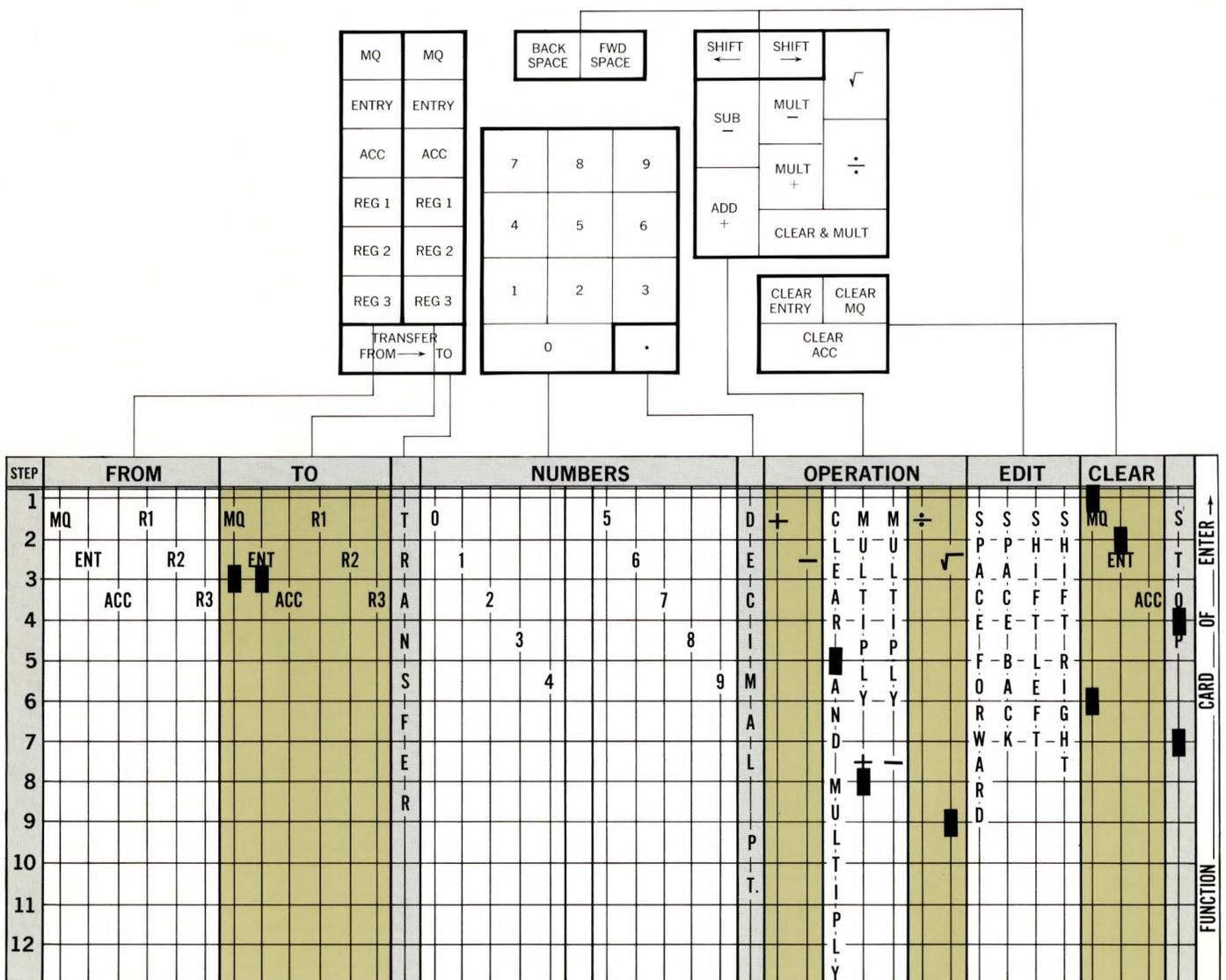
To program problems requiring more steps than are provided for on each card, you continue programming on additional cards. When you feed the prepared cards into PAC, the *Scientific* operates automatically until a "Stop" is
