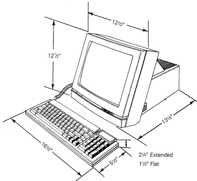
Ambient room temperature should never exceed 45 degrees Celsius (113 degrees Fahrenheit) when the terminal is on; however, the terminal needs no special cooling. Users should make sure the rear of the terminal has a free flow of air. They shouldn't set the terminal on sound-deadening devices that block the flow of air beneath it.
