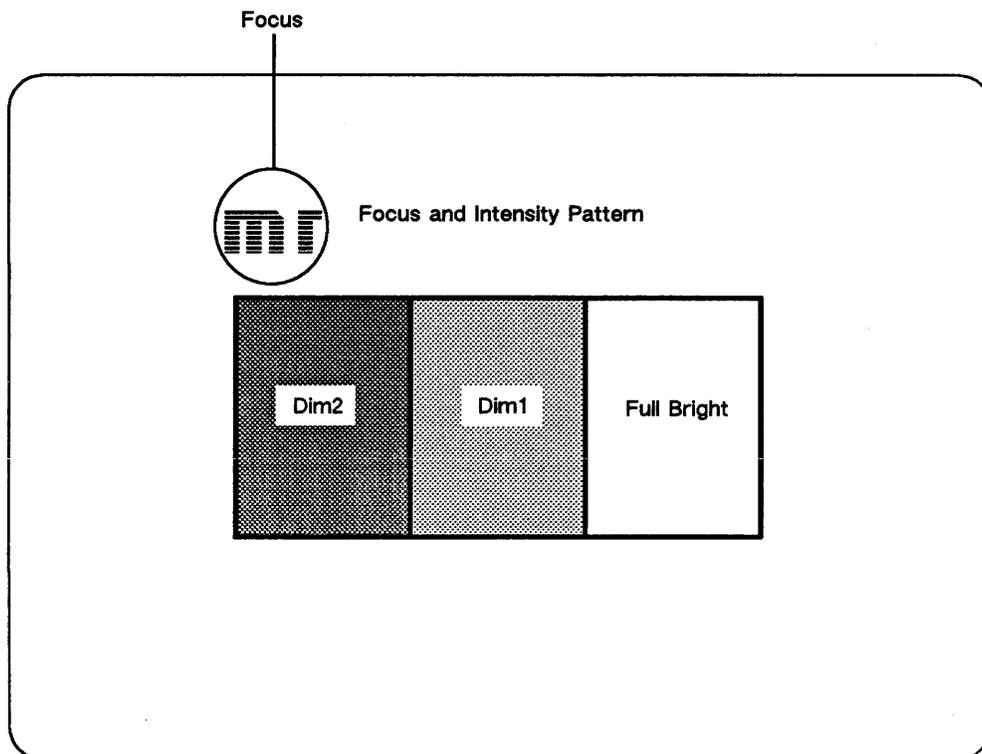
This pattern is an 80 or 132-column display of characters. (Hold the CTRL key and press the S key to toggle between 80 and 132 columns.) Three blocks in the center of the pattern indicate brightness: bright, normal, and dim.
