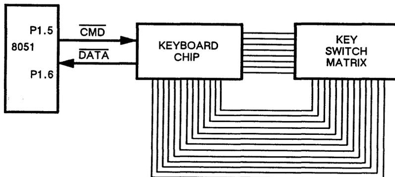
The keyboard PCB is arranged as a matrix of up to 13 rows of eight columns each. Each key switch connects one row to one column when that key is pressed. The keyscanner interface chip has 13 open-drain row outputs and eight column inputs with active pullups. The integrated circuit communicates with the external processor on two lines: the command line ( $\overline{\text{CMD}}$ ) and the data line ( $\overline{\text{DATA}}$ ).
