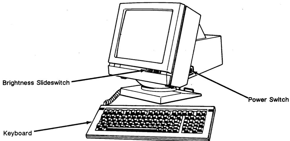
The power switch is on the right side of the terminal. Pressing the back of the switch turns AC power on.
