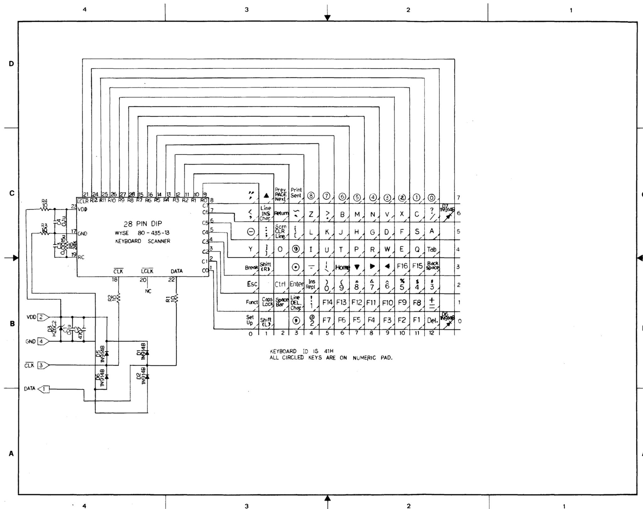
Figure 7-2 AT-Style Keyboard PCB Schematic
