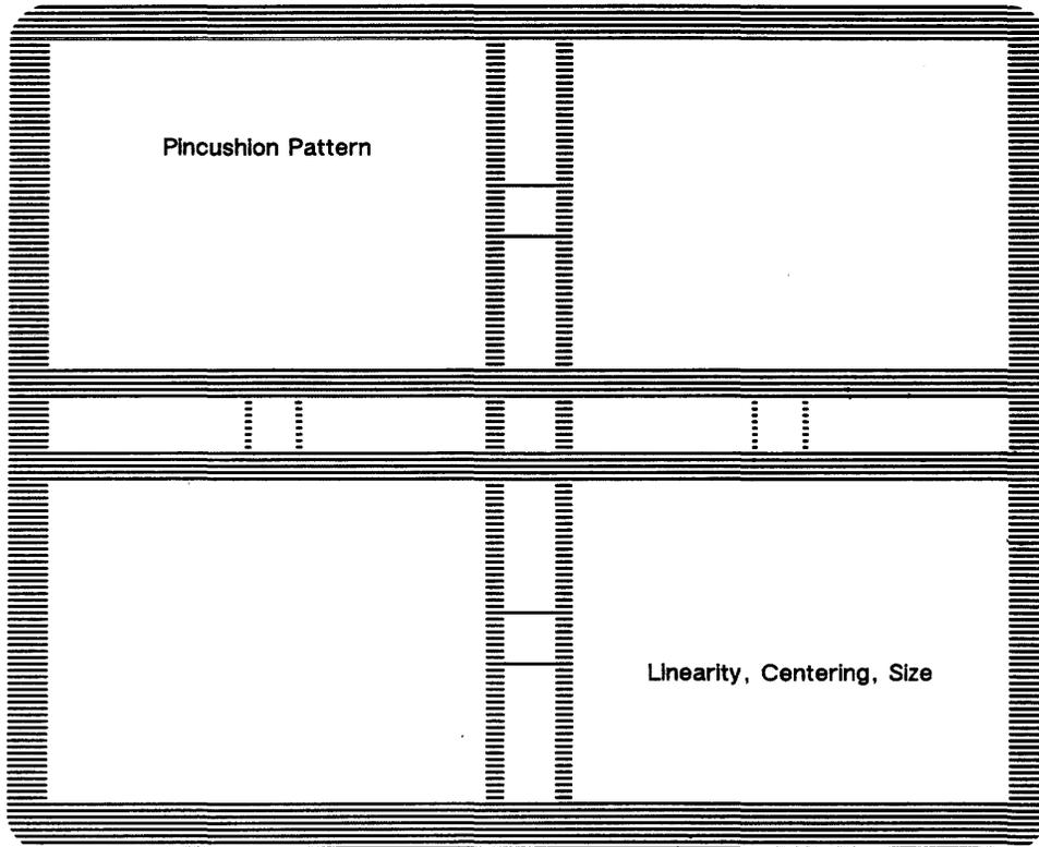
You can verify the display tolerances using both patterns along with a display reticle. See Appendix D for reticle instructions.
