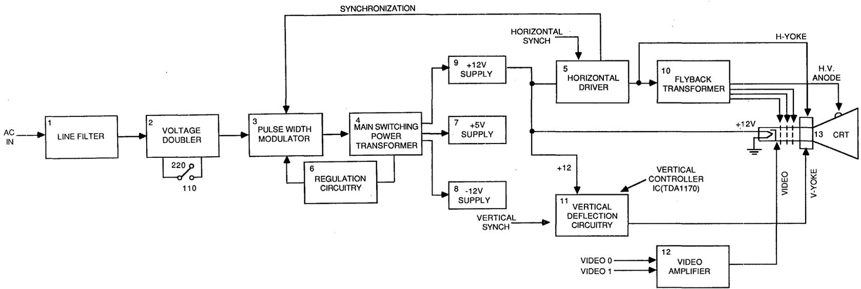
**-12 volt supply (8)**--The -12V supply is derived from one of the main transformer taps. The low voltage AC output is rectified and filtered. The -12 volt supply is  $V_{EE}$  for the RS-232 drivers.
