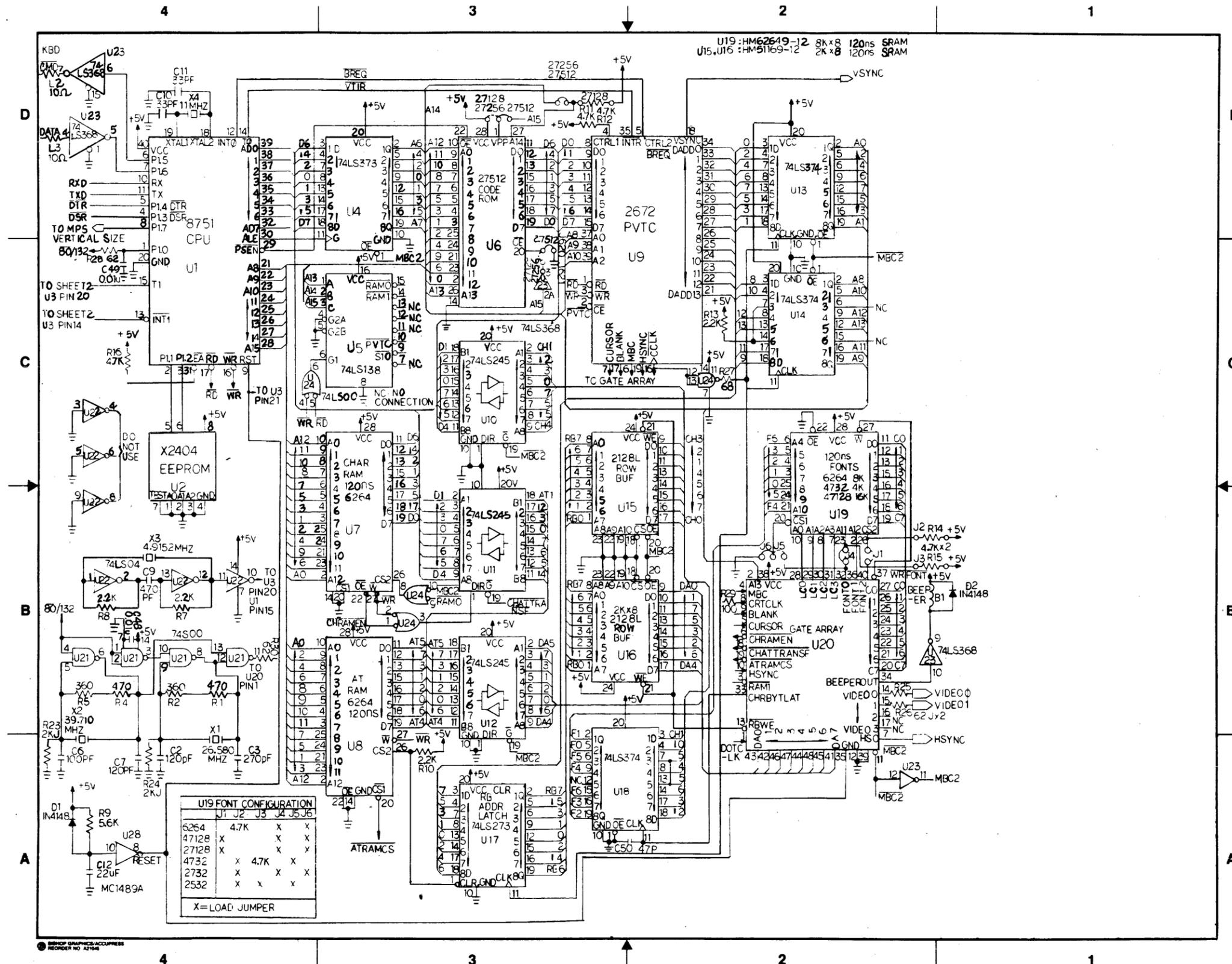
Figure 7-4 Terminal PCB Schematic (Monitor/Power Supply),
