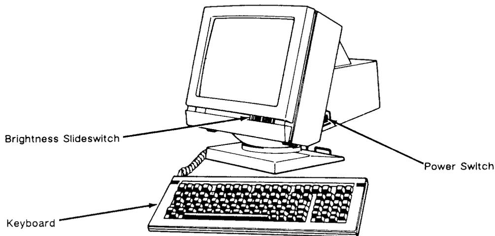
The power switch is on the right side of the terminal. Pressing the back of the switch turns AC power on.
