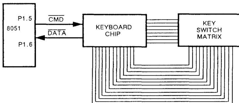
The keyboard PCB is arranged as a matrix of up to 13 rows of eight columns each. Each key switch connects one row to one column when that key is pressed. The keyscanner interface chip has 13 opendrain row outputs and eight column inputs with active pullups. The integrated circuit communicates with the external processor on two lines: the command line ( $\overline{CMD}$ ) and the data line (DATA).
