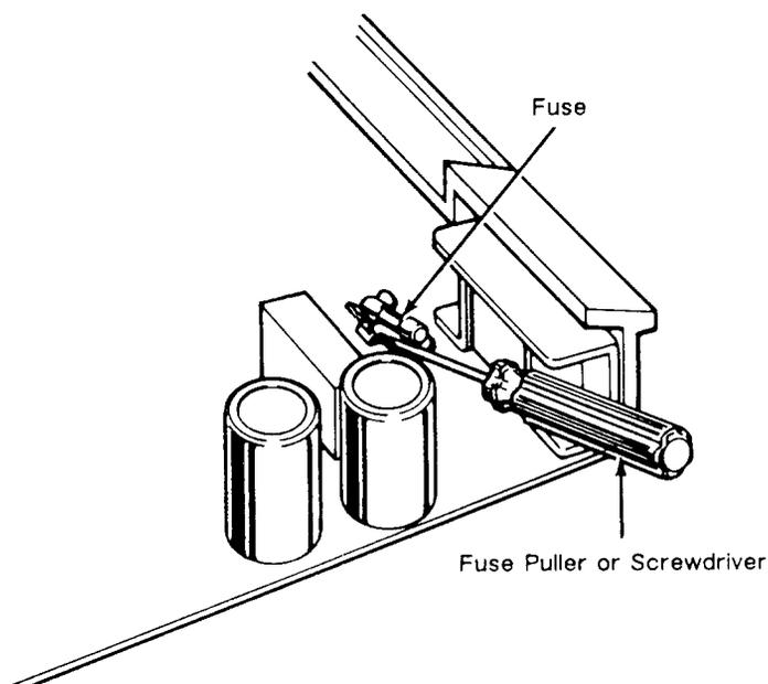
3. Check the fuse. If the fuse is broken or blackened, push a new fuse into the fuse socket.
