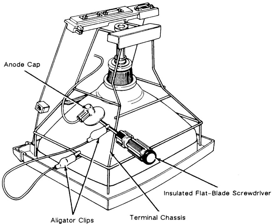
4. Slip the blade between the anode cap and the anode. Touch the blade to the wire anode leads under the cap. Listen for a popping or crackling sound.
