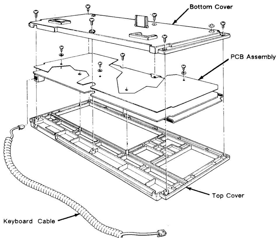
5. Remove the No. 0 Phillips screw beneath the SPACEBAR that holds the keyboard top cover to the PCB assembly.
