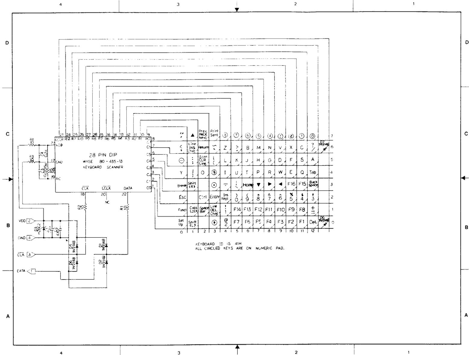
Figure 7-1 WY-60 ASCII Keyboard PCB Schematic
