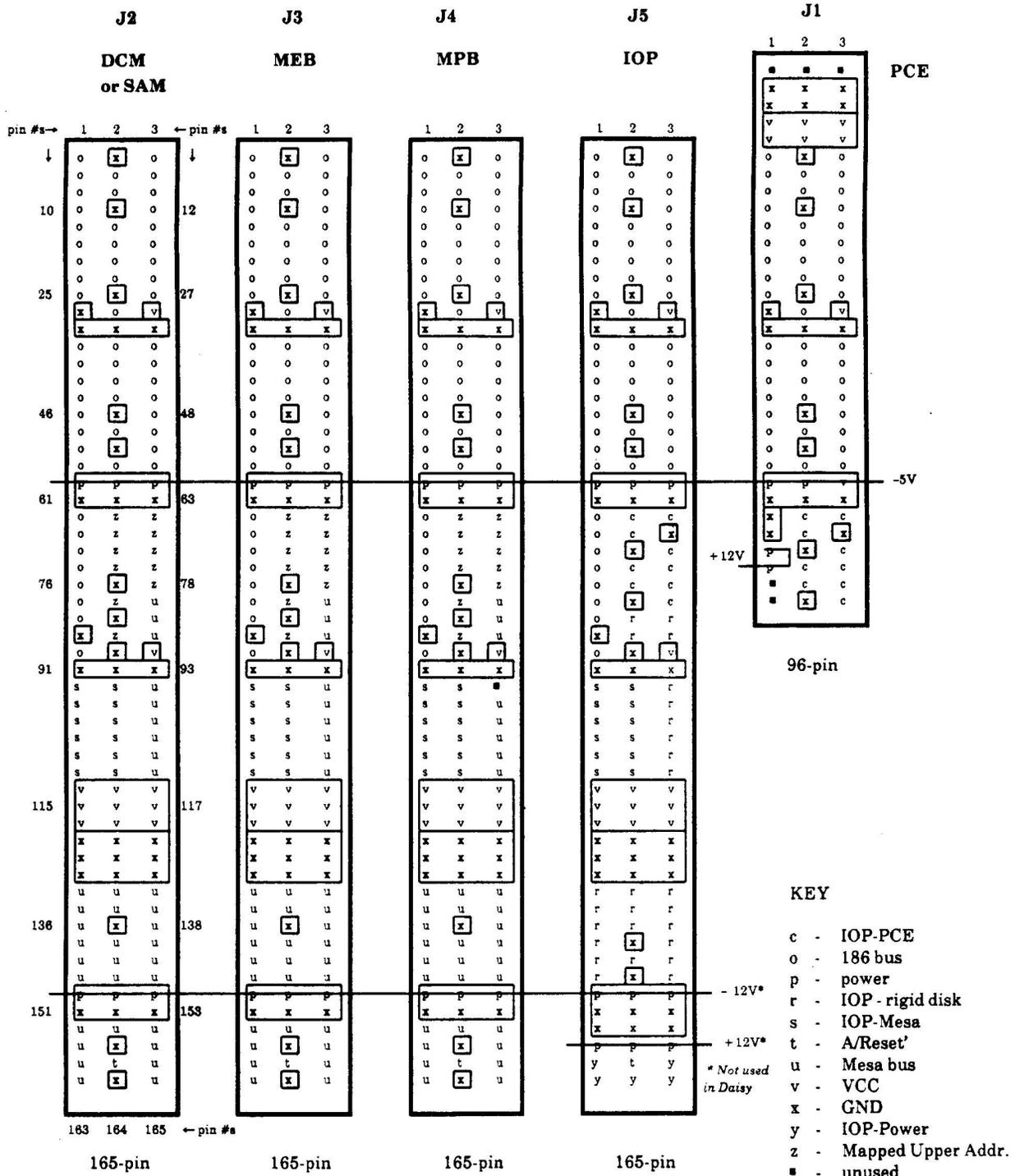
Figure 1.4. Signal flow of 165-pin connectors (front view)
