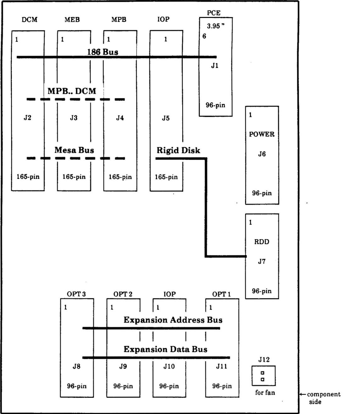
Figure 1.3. Bus routing (logic board side)
