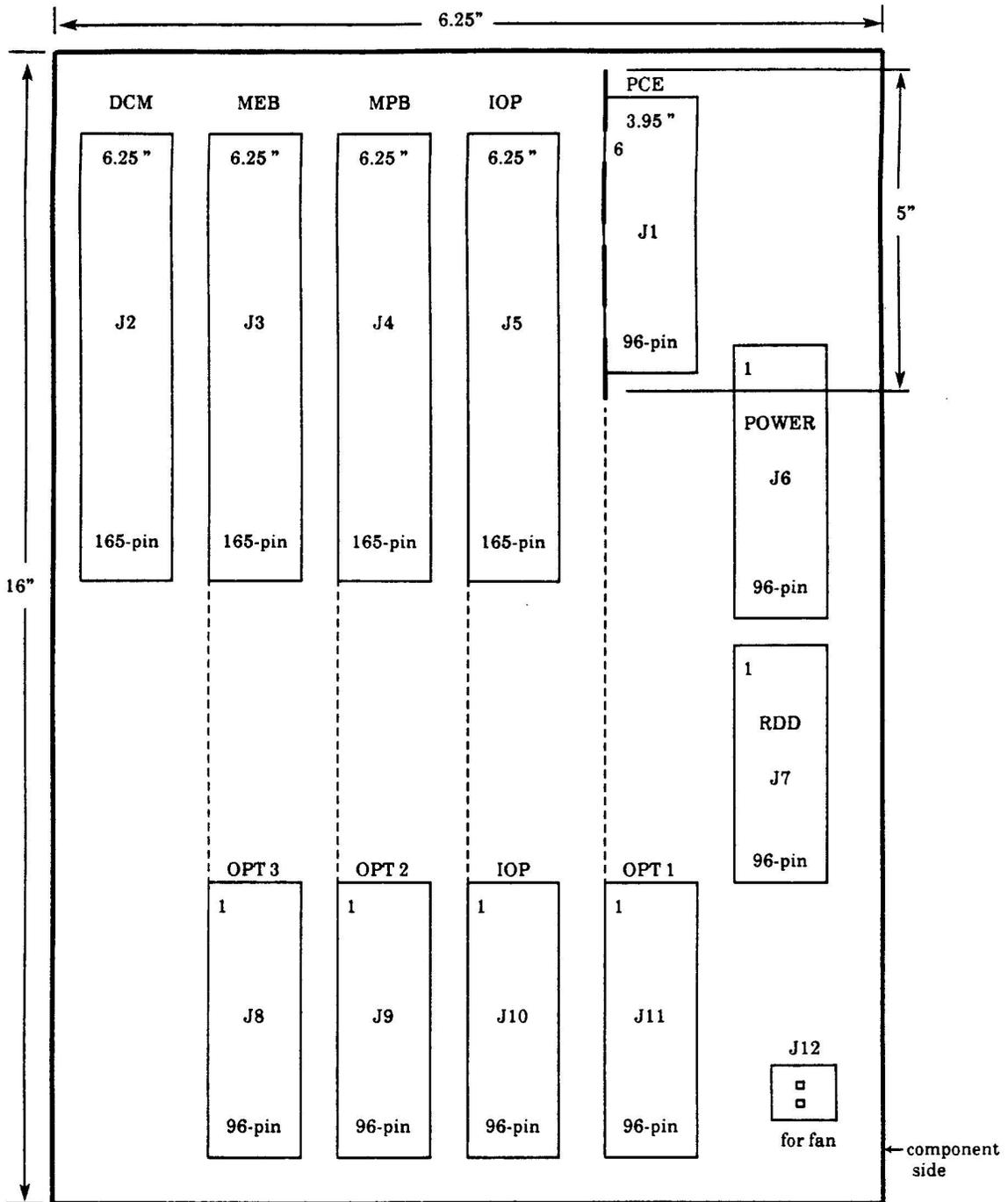
Figure 1.2. Backplane from logic board side
