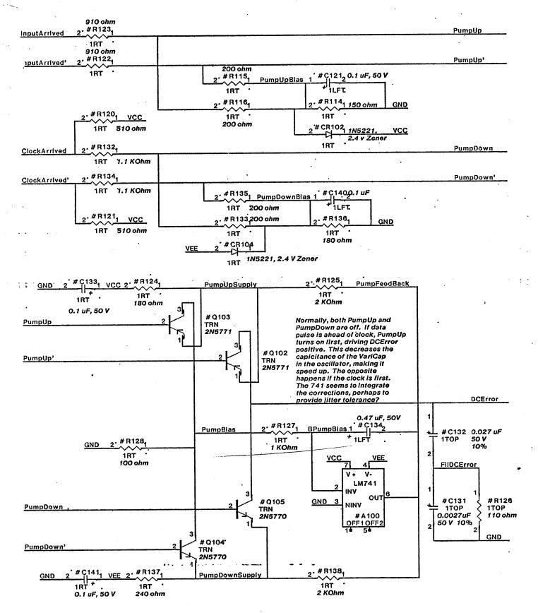
"Il resistors shown are 0.25 watt, 5% parts. All capcitors shown on this page have 10% tolerances.
