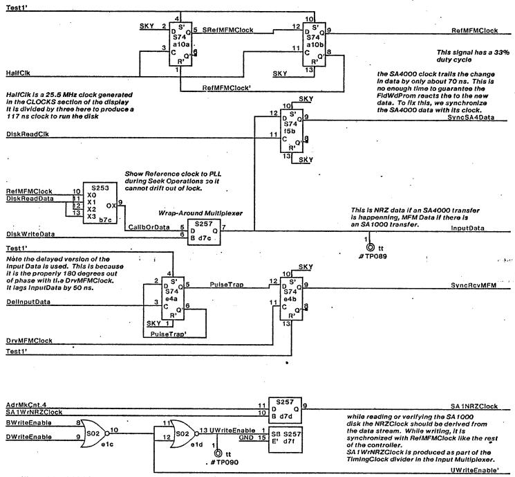
We note that AdrMkCnt.4 ceases to be active when TransferEnable drops. A clock is needed to start a write operation, so SA1NRZClock is set to the always active SA1WrNRZClock as soon as WriteEnable goes active. To ensure the DWriteEnable shift regiter delay is cleared, we keep SA1NRZClock set to SA1WrNRZClock until DWriteEnable goes to.
