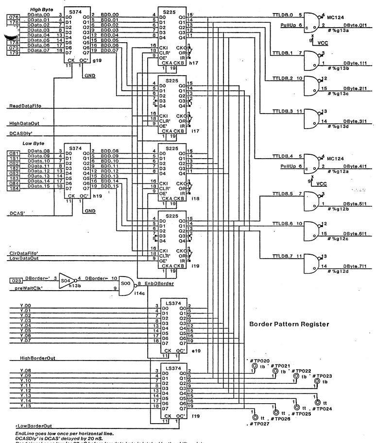
Read signal goes low for 20 nS before low data byte is latched by the shift register. Project **XEROX** Data FIFO and File Designer Rev Date Page SDD Border Register WS HS1025.sil Crane Q 6/21/80 25 STATES AND STATES AND STATES Control of the second of the
