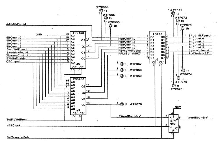
Using an S74 instead of the LS273 speeds up WordBoundry' so it will change before the RawCRCError indicator from the 9401 CRC Checker. This allows us to latch the CRCError signal directly using WordBoundry'. The RawCRCError signal is too slow to latch into the Word Status buffer register using NRZClock'. There is then a race between WordBoundry' and RawCRCError after NRZClock rises. Using the faster S74 here ensures WordBoundry' wins.
