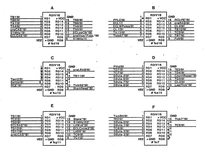
Termination Packages A, B, C, D, E above are 100 ohm termination to -2 V
