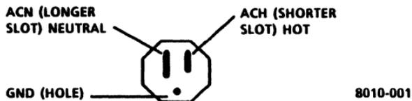
Figure 6-4 USO AC Outlet at Wall
