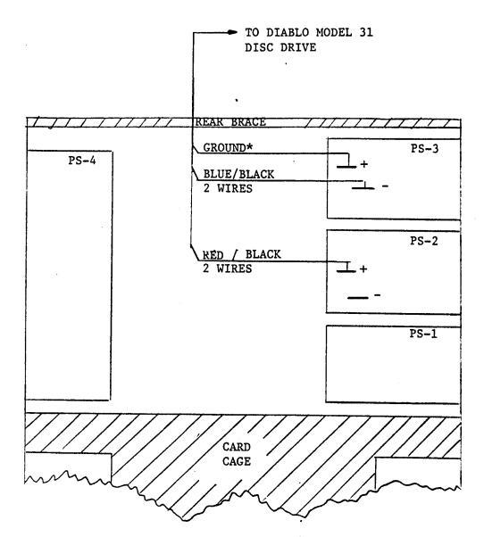
\*NOTE: GROUND WIRE MAY BE EITHER A BARE WIRE OR A BARE WIRE WITH BLACK SHRINK TUBING ON IT.
