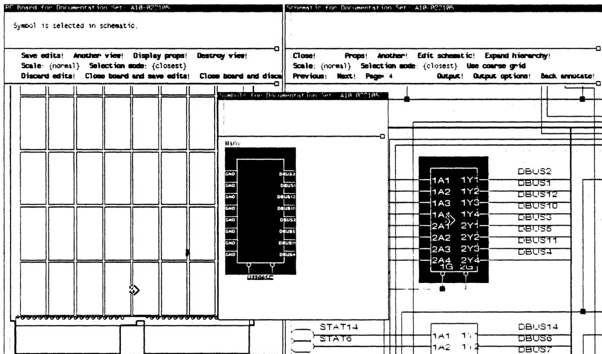
Cross-Reference from PC Board to Schematic
