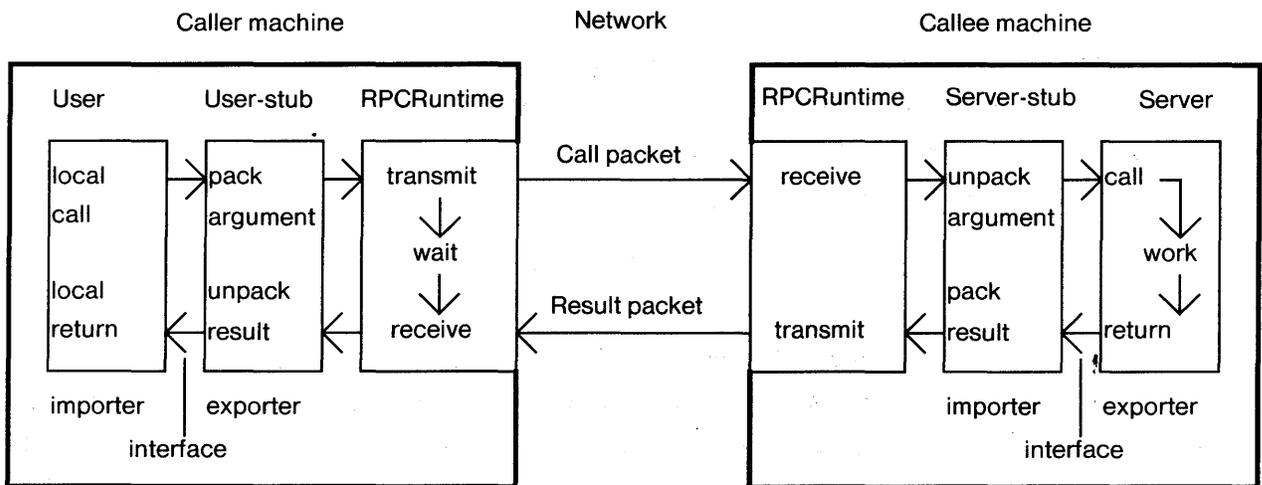
**Figure 1:** The components of the system, and their interactions for a simple call.
