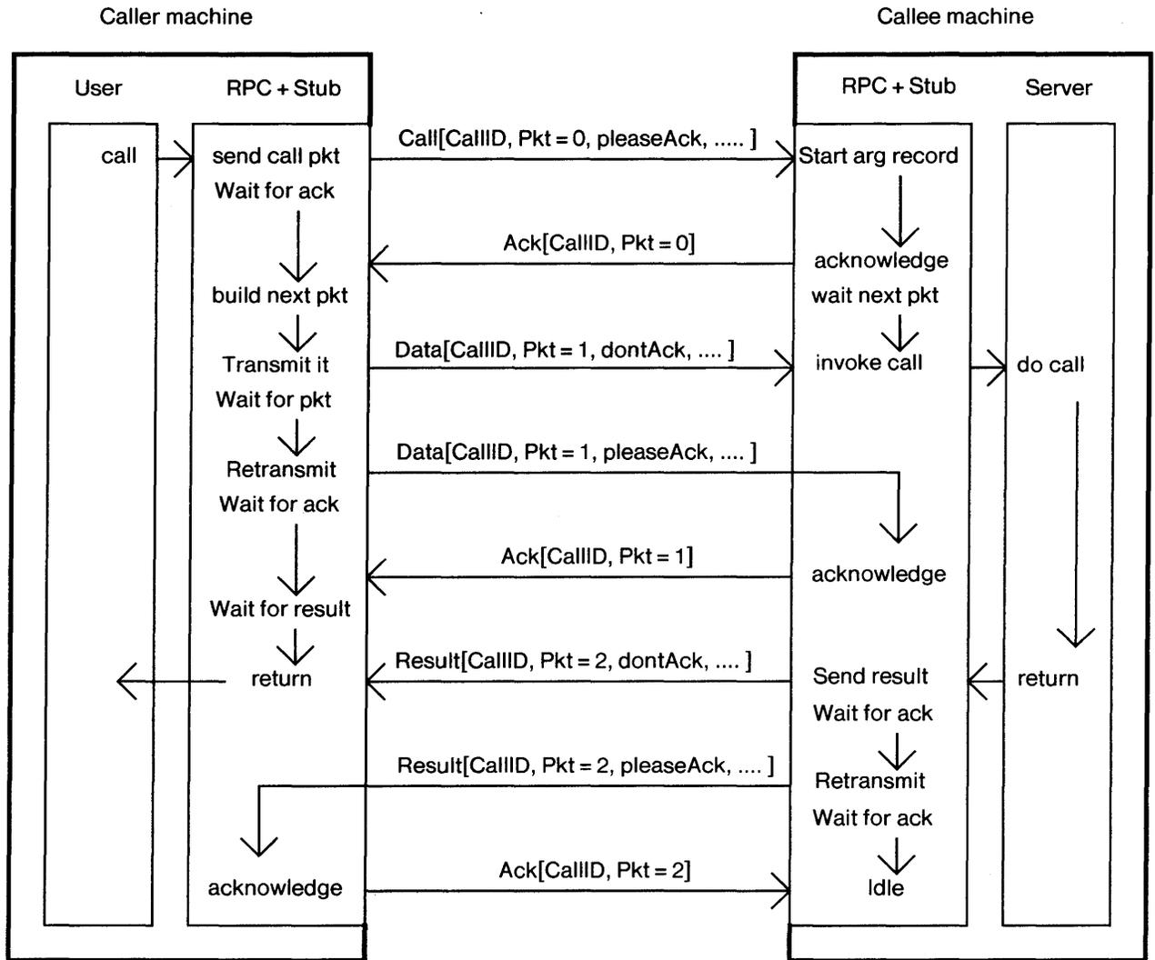
**Figure 4:** A complicated call. The arguments occupy two packets. The call duration is long enough to require retransmission of the last argument packet requesting an acknowledgement, and the result packet is retransmitted requesting an acknowledgement because no subsequent call arrived.
