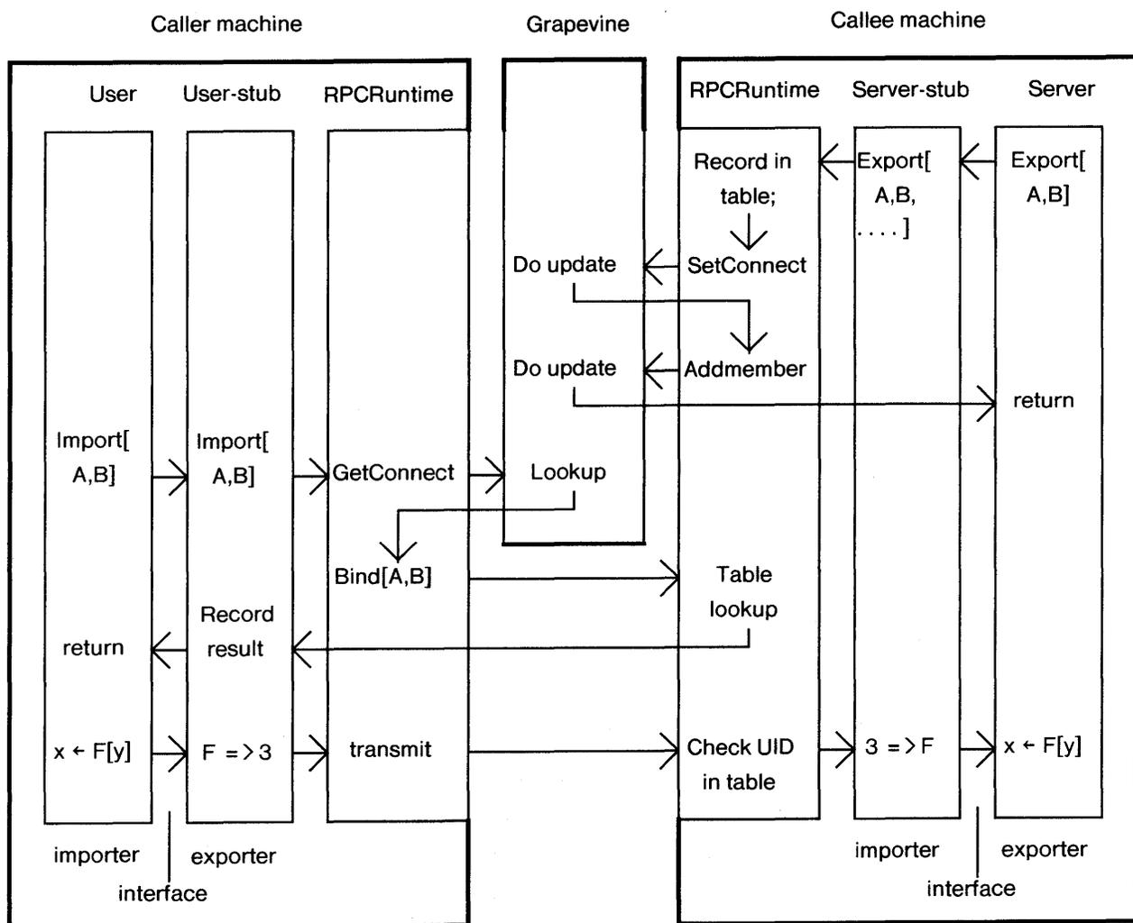
**Figure 2:** The sequence of events in binding and a subsequent call. The callee machine exports the remote interface with type "A" and instance "B". The caller machine then imports that interface. Then we show the caller initiating a call to procedure "F", which is the third procedure of that interface. The return is not shown.
