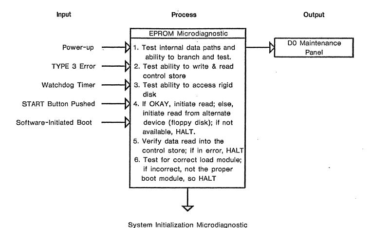
1. The major goal of this microdiagnostic is to check the load path between the control store and the system load device so that the System Initialization Microdiagnostic can be loaded without errors.
