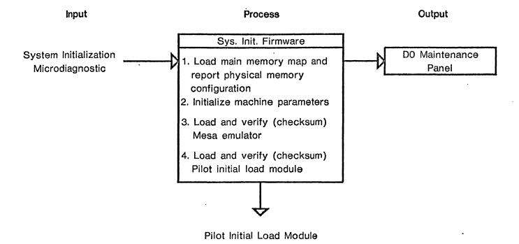
1. Data obtained during the boot operation will tentatively be stored in main memory in locations known to Pilot. The amount of information so saved will be limited to indicating the cause of the boot operation, summary information on non-critical errors encountered (not: critical errors will cause the boot operation to HALT), and main memory map data.
