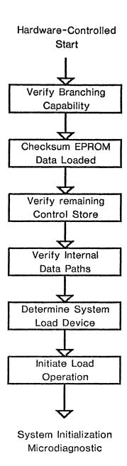
Figure 5. EPROM Microdiagnostic, HIPO Structure Diagram
