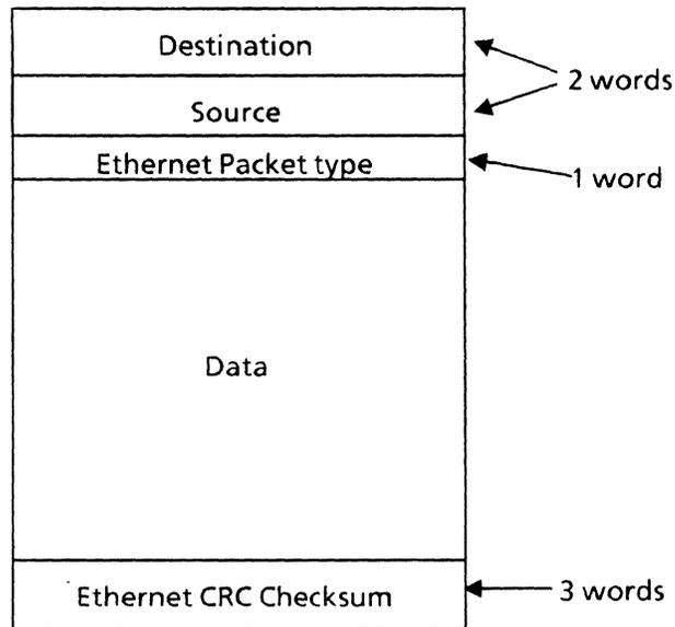
Figure 2.5 Ethernet packet
